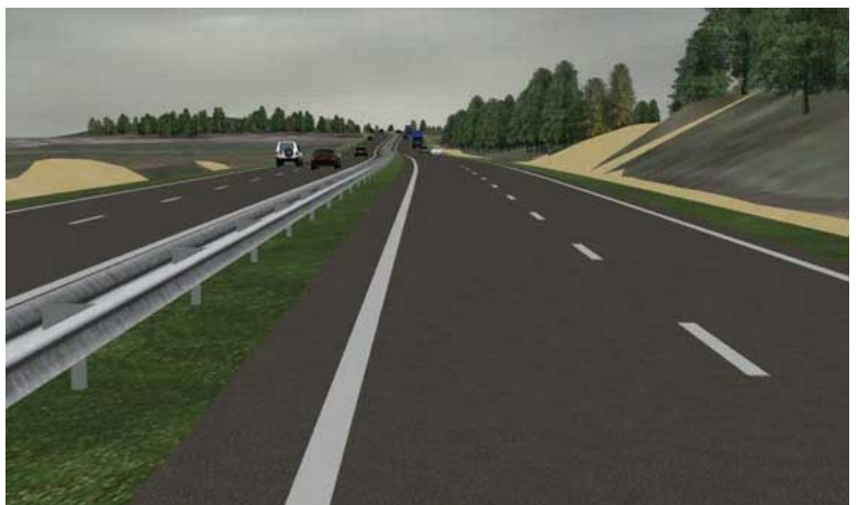
Figure 2 - Arup uses visualization techniques to identify potential safety concerns on proposed highway alignments. Image courtesy of Arup.
