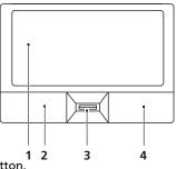
Use Acer Bio-Protection fingerprint reader (3) supporting Acer FingerNav 4-way control function (only for certain models) to scroll up or down and move left or right a page. This fingerprint reader or button mimics your cursor pressing on the right scroll bar of Windows applications.
