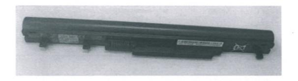
J-ion Battery Pack (電腦/电压) Rating: 14.8V === (容量/容量) 3000mAh, 44Wh type. Dispose of used batteries according to the Instructions. release toxic materials. Do not short circuit; may cause burns. 联络。使用其他电池替换,将可能引起安全问题。
