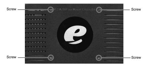
**8** Attach the adjustable stand's mounting flange to the LCD panel using the four screws you removed.
