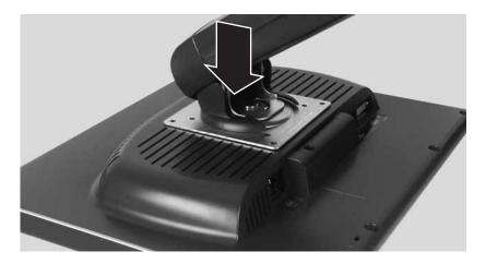
**9** Use the four large screws provided with the adjustable stand to attach the base to the adjustable stand. Insert the screws through the bottom of the base and into the stand's neck.
