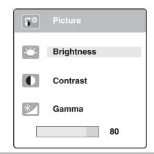
**Brightness**—Adjusts the amount of light in the darkest portion of the picture. Use the lowest brightness setting you are comfortable with to maximize the life of the monitor backlights.
