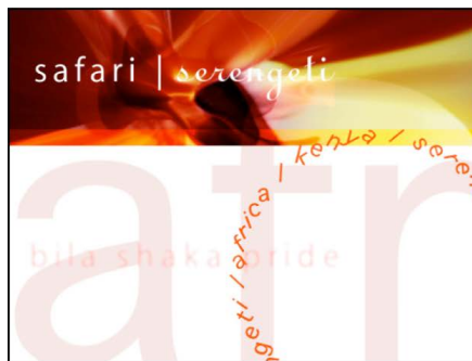
Spin behavior applied to text on a path with Affect Subobjects turned on (the individual text characters spin)
