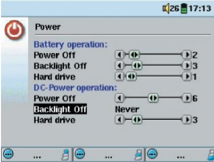
You can set the AV300 to conserve power for both modes of operation (when it is powered from the battery, or when it is connected to the AC charger/adaptor (DC-Power operation)).
