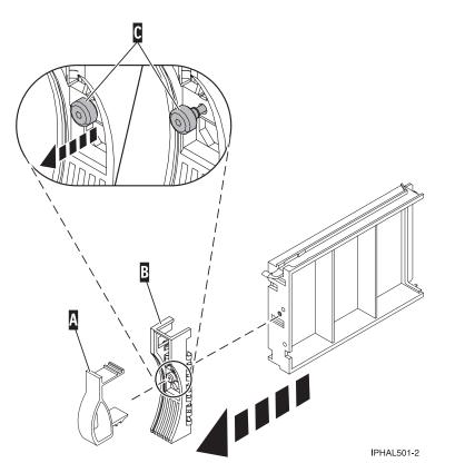
Figure 42. Removing a disk-drive bezel
