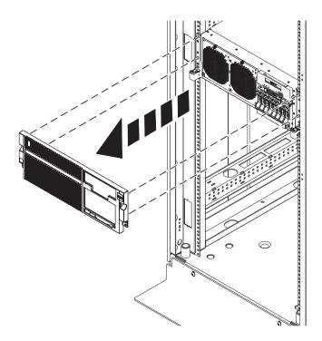
Figure 91. Removing the front cover
