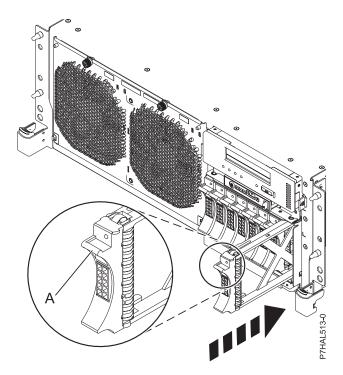
Figure 41. Installing a disk drive filler in the system
