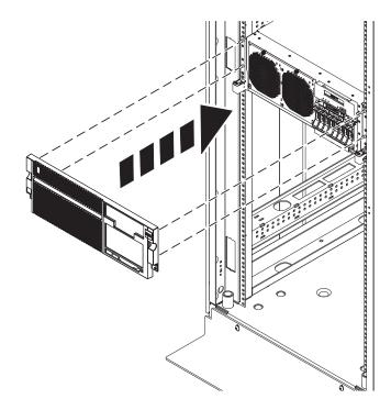
Figure 93. Removing the front cover
