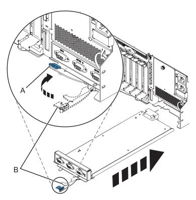
Figure 71. Replacing the enclosure management controller
