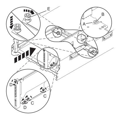
Figure 69. Installing the SAS conduit card and the midplane
