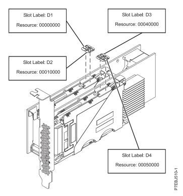
Figure 44. PCIe RAID and SSD SAS adapter locations
