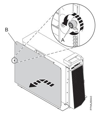
Figure 97. Installing the outside service access cover
