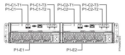
Figure 57. Rear view of the 58/87 disk drive enclosure
