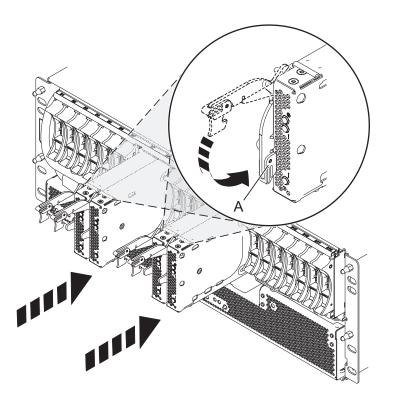
Figure 85. Installing the SAS expander card
