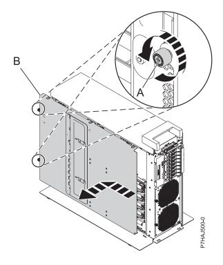
Figure 98. Removing the inside service access cover
