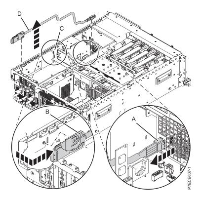
Figure 37. Removing the external SAS port
