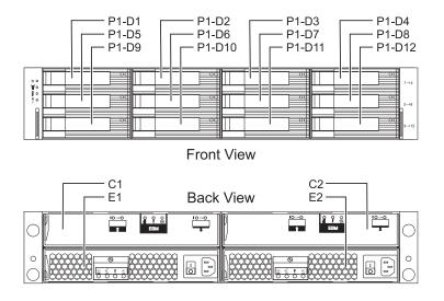
Figure 54. Disk drive locations for the 58/86 disk-drive enclosure
