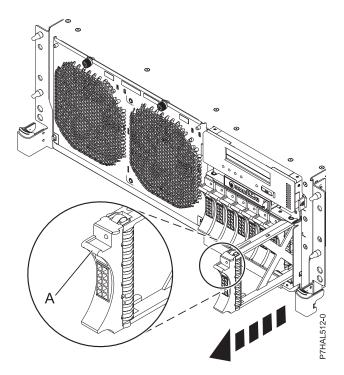
Figure 40. Removing a disk drive filler from the server
