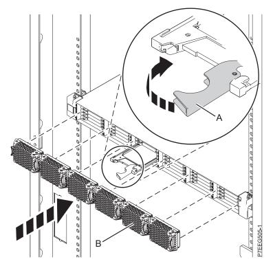
Figure 14. Installing a solid-state drive in the ED/R1 PCIe storage enclosure
