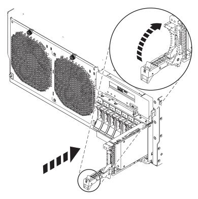
Figure 6. Installing the disk drive in the system
