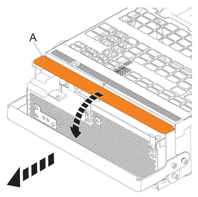
Figure 79. Remove the offline converter assemblies
