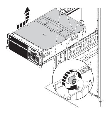
Figure 96. Removing the service access cover
