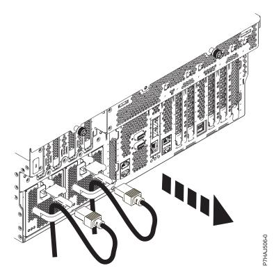
Figure 106. Removing the power cords for a rack-mounted system
