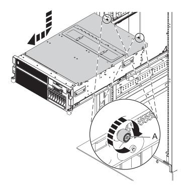
Figure 99. Installing the service access cover
