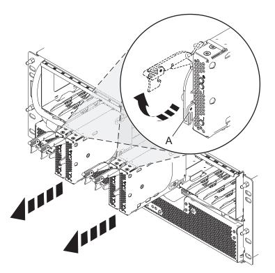
Figure 86. Removing the SAS expander card.
