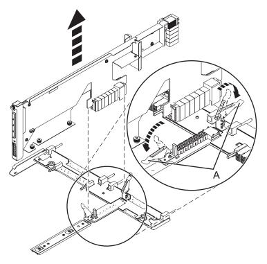
Figure 84. Removing the SAS conduit card from the midplane
