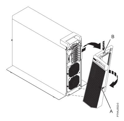
Figure 92. Removing the front cover
