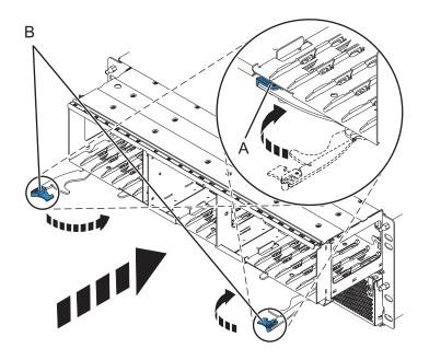
Figure 74. Installing the backplane on a rack-mounted model
