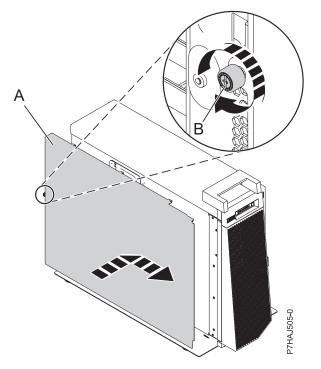
Figure 101. Installing the outside service access cover
