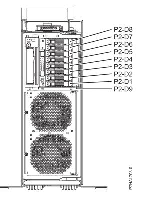
Figure 46. Disk drive locations for the stand-alone systems
