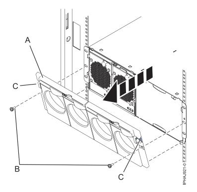
Figure 89. Remove the front cover for model 14G/30
