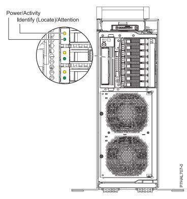
Figure 48. Service indicator locations for the stand-alone system
