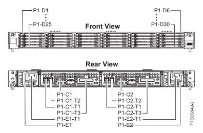
Figure 59. Front view and rear view of the 58/88 PCIe storage enclosure showing the solid-state drive locations
