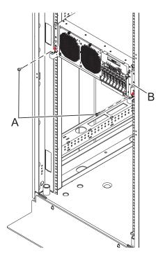
Figure 102. Placing the system unit in the service position
