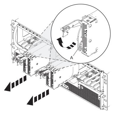
Figure 76. Removing the port card from the backplane
