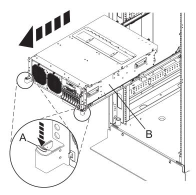
Figure 103. Locking the system unit in the service position
