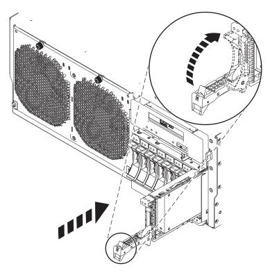
Figure 34. Replacing a disk drive or solid-state drive in the system
