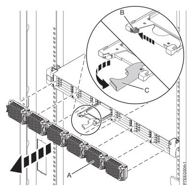
Figure 23. Removing the solid-state drive from the ED/R1 PCIe storage enclosure
