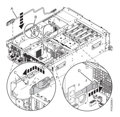
Figure 39. Replacing the SAS cable
