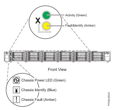
Figure 62. Front view of the ED/R1 PCIe storage enclosure showing the service indicators
