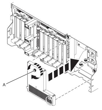
Figure 70. Installing the power cord plate
