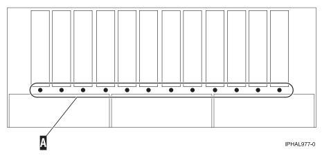
Figure 52. Front view of service indicators for 31D/24, and 31T/24
