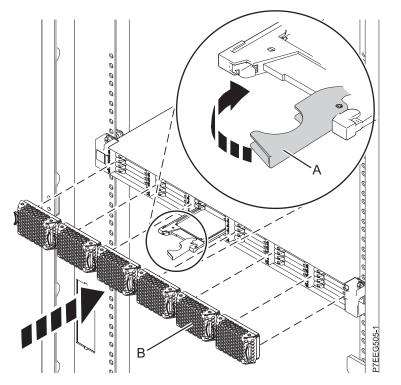
Figure 29. Replacing a solid-state drive in the ED/R1 PCIe storage enclosure.
