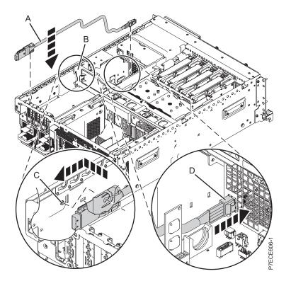
Figure 38. Installing the external SAS port
