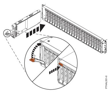
Figure 12. Installing the disk drive in the 58/87 disk drive enclosure
