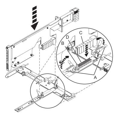
Figure 68. Installing the SAS conduit card into the midplane
