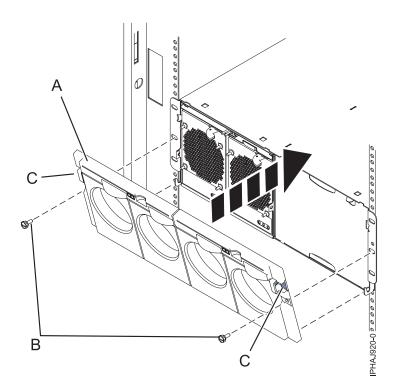
Figure 90. Front cover on a model 14G/30
