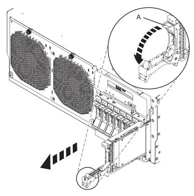
Figure 24. Removing a disk drive from the system
