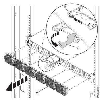
Figure 22. Removing the solid-state drive from the 58/88 PCIe storage enclosure
