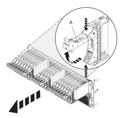
Figure 75. Removing the drives from the backplane
