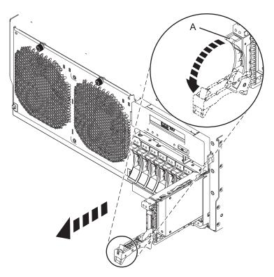
Figure 21. Removing a disk drive from the system
