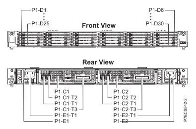
Figure 61. Front view and rear view of the ED/R1 PCIe storage enclosure showing the solid-state drive locations
