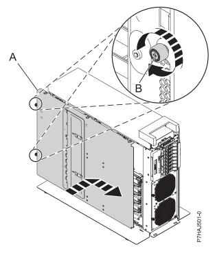
Figure 100. Installing the inside service access cover
