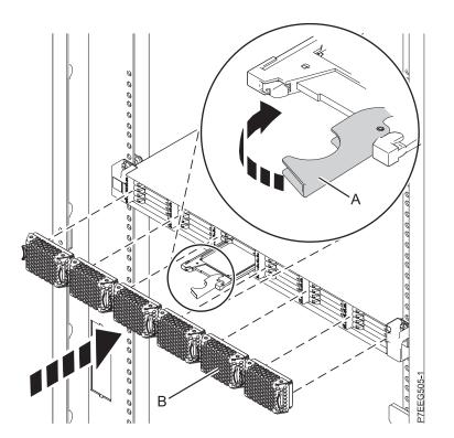
Figure 28. Replacing a solid-state drive in the 58/88 PCIe storage enclosure.
