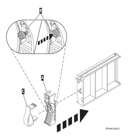
Figure 43. Attaching a bezel to a disk drive filler
