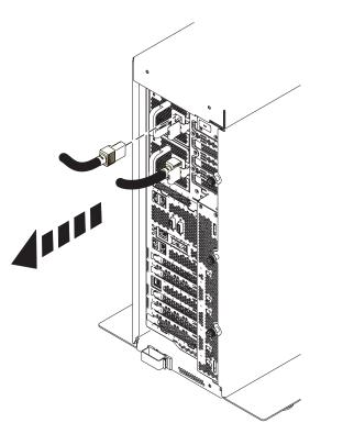
Figure 107. Removing the power cords for a stand-alone system
