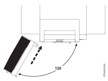
Figure 95. Installing the front door
