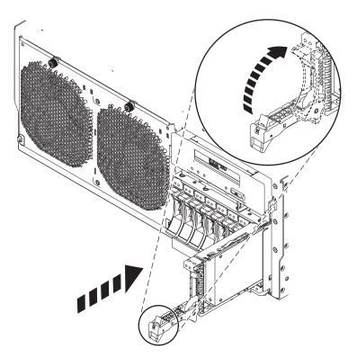
Figure 11. Installing the disk drive in the system
