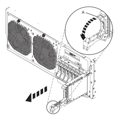
Figure 15. Removing a disk drive from the system
