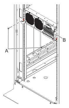
Figure 105. Placing the system unit into the operating position
