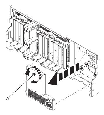
Figure 81. Removing the power cord plate
