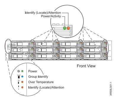
Figure 55. Front view of disk drive enclosure service indicators for the 58/86
