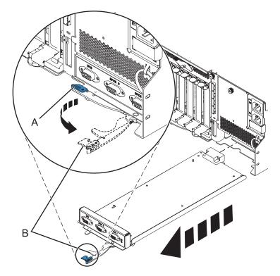
Figure 80. Remove the enclosure management controller
