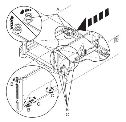
Figure 83. Removing the SAS conduit card and midplane
