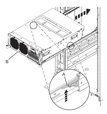
Figure 104. Placing the system unit into the operating position
