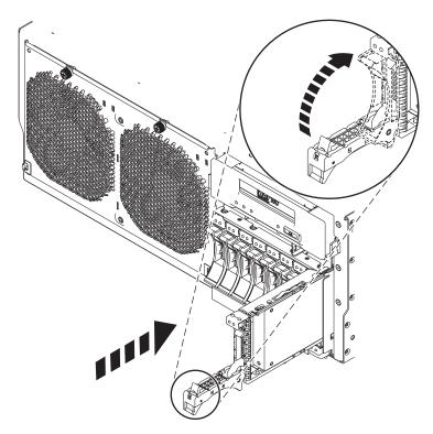
Figure 31. Replacing a disk drive in the system
