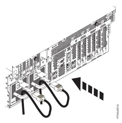
Figure 108. Connecting the power cords
