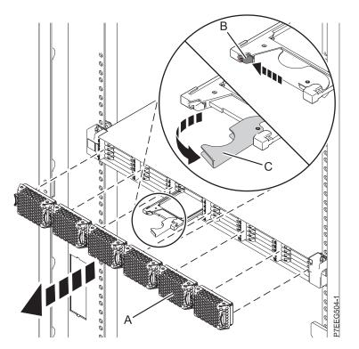
Figure 25. Removing the solid-state drive from the 58/88 PCIe storage enclosure
