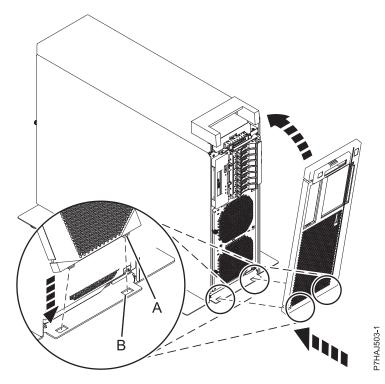
Figure 94. Installing the front cover
