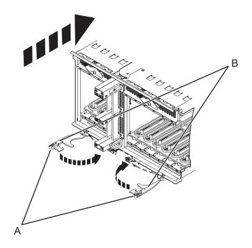
Figure 72. Install the I/O system board on a rack-mounted model
