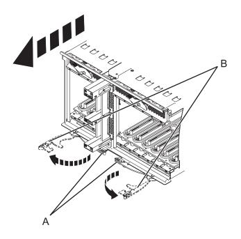
Figure 82. Removing the I/O system board
