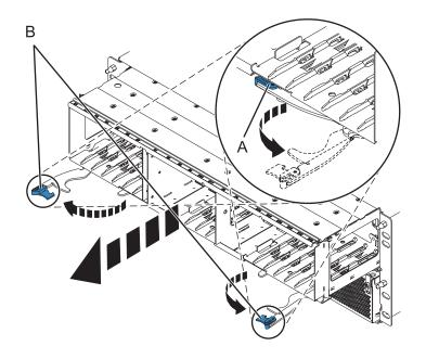
Figure 77. Removing the backplane from the enclosure
