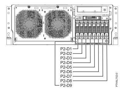
Figure 45. Disk drive locations for the rack-mounted systems
