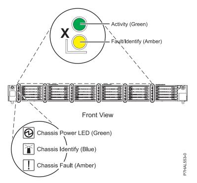
Figure 60. Front view of the 58/88 PCIe storage enclosure showing the service indicators
