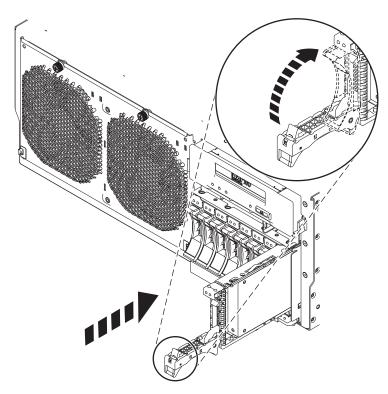
Figure 27. Replacing a disk drive in the system
