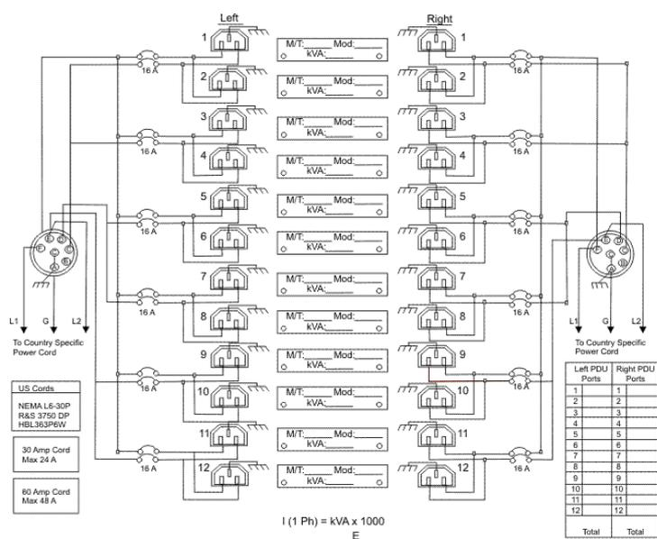
PDU load sequence schematic
