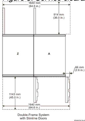
The minimum service clearance for systems with acoustical doors is shown in the following figure.
