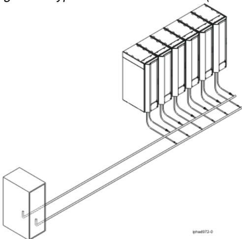
**Flexible hoses and connections to manifolds and heat exchangers**
