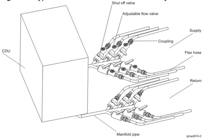
The following figure shows another layout for multiple water circuits.
