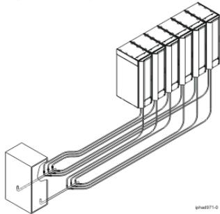
The following figure shows an extended manifold layout.
