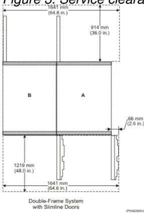
The minimum service clearance for systems with acoustical doors is shown in the following figures.
