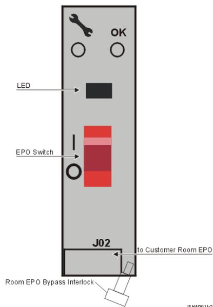
When the switch is reset, the utility power is confined to the system power compartment. All volatile data will be lost.
