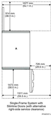
The minimum service clearance for systems with acoustical doors is shown in the following figures.
