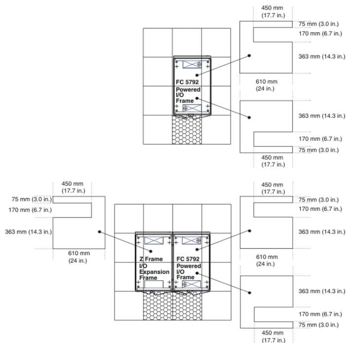
**Note:** This figure shows a dual frame configuration. If your installation uses a single frame configuration, use the dimensions associated with the primary frame.
