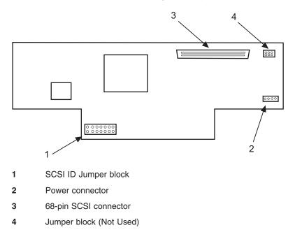
Rear View of the SCSI-to-IDE Interface Bridge for Optical Devices
