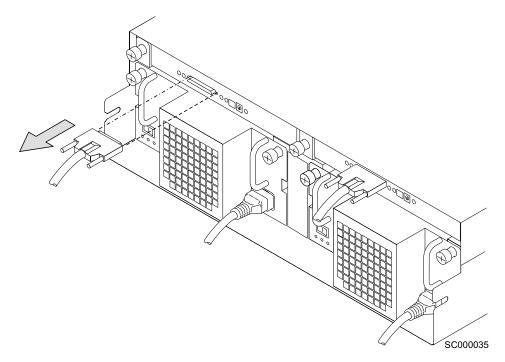
Figure 69. Removing the SCSI cable
