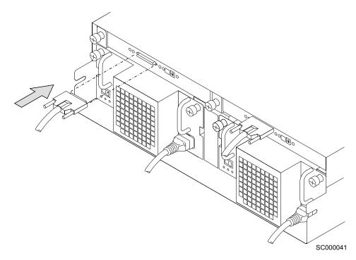
Figure 77. Plugging in the SCSI cable
