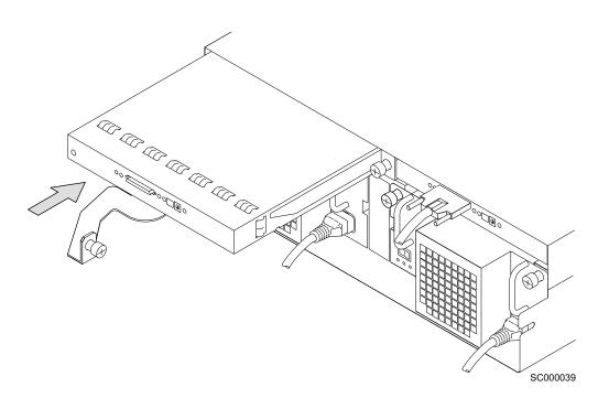
Figure 74. Pushing the replacement SCSI Interface card in
