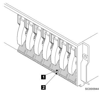
Figure 48. Disk drive module lights
