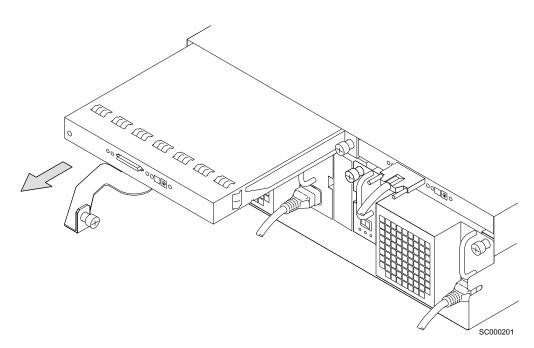
Figure 72. Pulling the SCSI Interface card out
