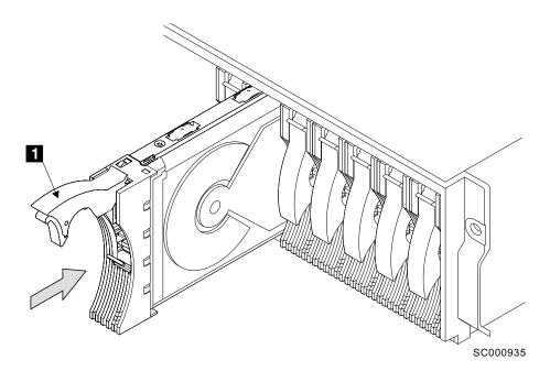
Figure 38. Adding a disk drive module
