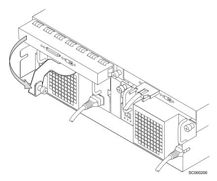
Figure 71. Opening the lever
