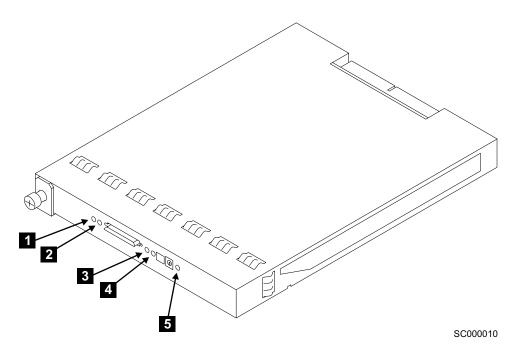
Figure 28. SCSI Interface card assembly lights
