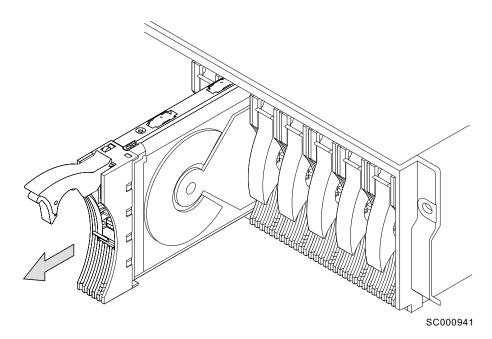
Figure 45. Removing a disk drive module
