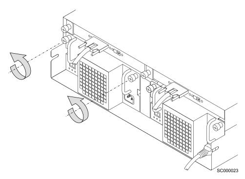
Figure 53. Unscrewing the thumbscrews on the fan-and-power-supply assembly
