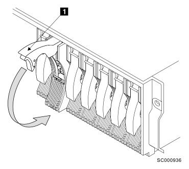
Figure 39. Closing the handle of a disk drive module
