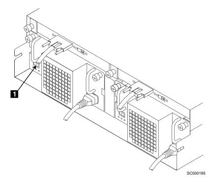
Figure 51. Fan-and-power-supply dc on/standby switch
