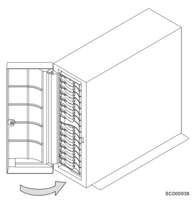
Figure 41. Closing the cover of a 2104 Model TS4
