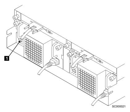
Figure 58. Fan-and-power-supply dc on/standby switch
