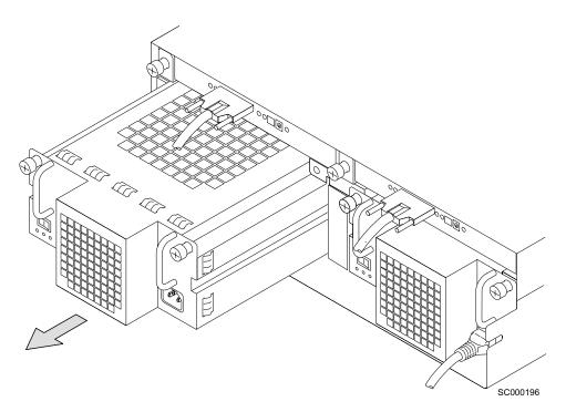
Figure 54. Removing the fan-and-power-supply assembly
