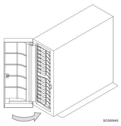
Figure 49. Closing the cover of a 2104 Model TS4
