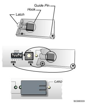
Figure 73. Inside of the switch cover plate showing the hook, latch, and two guide pins to mate with the SCSI Interface card assembly
