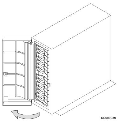
Figure 43. Disk drive modules in a 2104 Model TS4
