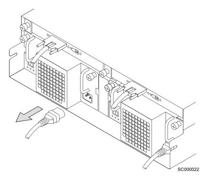
Figure 52. Unplugging the mainline power cable
