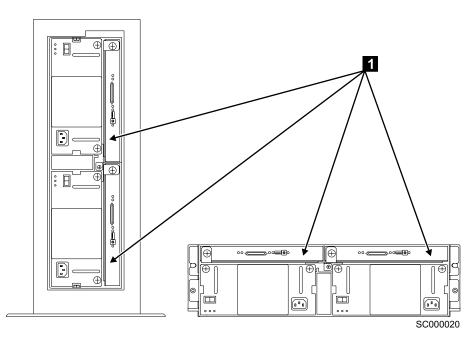
Figure 27. SCSI Interface cards in a 2104 Model TS4 (left) and 2104 Model DS4 (right)
