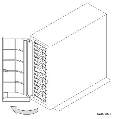
Figure 36. Disk drive modules in a 2104 Model TS4
