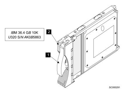
Figure 34. Disk drive module handle and label (2104 Model DS4 or Model TS4)
