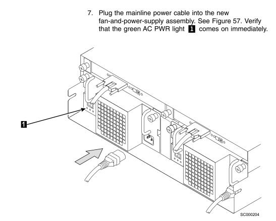
Figure 57. Plugging in the mainline power cable
