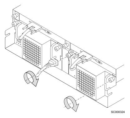
Figure 65. Tightening the thumbscrews
