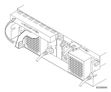
Figure 75. Closing the lever
