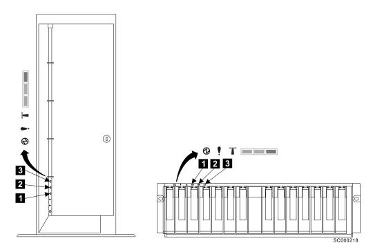
Figure 21. Disk enclosure lights on a 2104 Model TS4 (left) and a 2104 Model DS4 (right)
