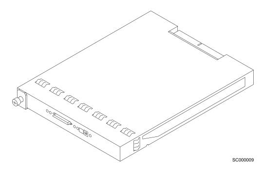
Figure 67. SCSI Interface card assembly
