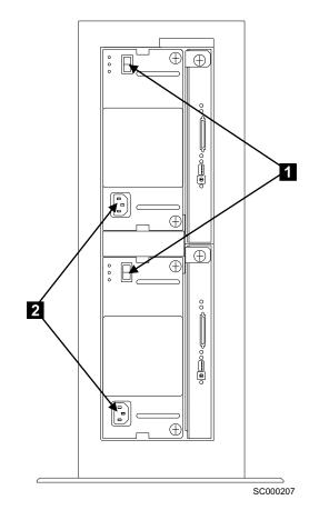
Figure 11. Removing power from a 2104 Model TS4
