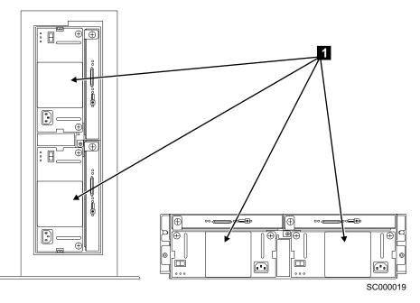
Figure 24. Fan-and-power-supply assemblies in a 2104 Model TS4 (left) and 2104 Model DS4 (right)
