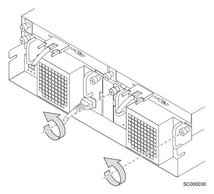
Figure 62. Unscrewing the thumbscrews on a fan assembly
