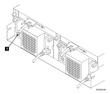
Figure 50. A fan-and-power-supply assembly
