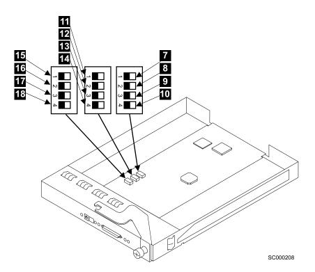
Figure 30. Other switches on the SCSI Interface card
