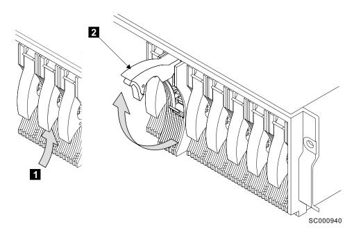
Figure 44. Opening the disk drive module handle
