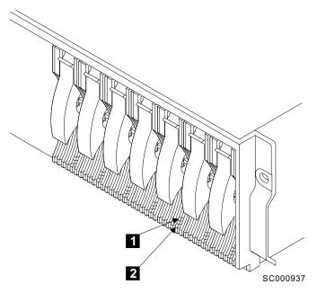
Figure 40. Disk drive module lights
