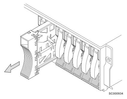
Figure 37. Removing a dummy disk drive module
