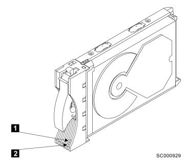
Figure 23. Disk drive module lights
