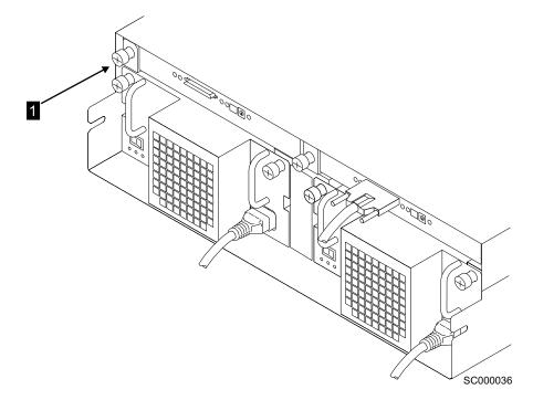
Figure 70. Unscrewing the SCSI Interface card
