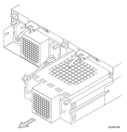
Figure 63. Pulling out a fan assembly
