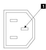
Figure 9. Ground pin (2104 Model TS4)
