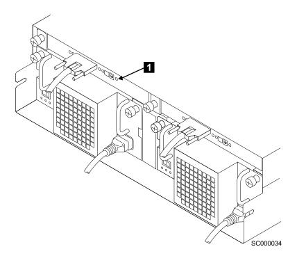
Figure 68. Fault light on an SCSI Interface card assembly
