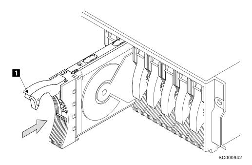
Figure 46. Inserting a disk drive module
