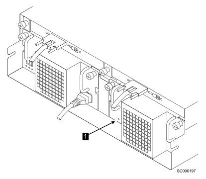
Figure 66. Fan assembly light
