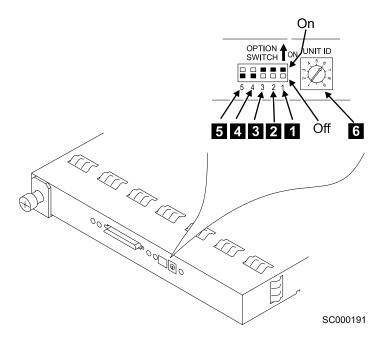
Figure 29. SCSI Interface card switches
