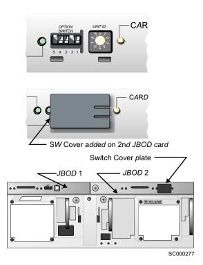
Figure 31. Switch cover plate on the panel of the SCSI Interface card-2 (second JBOD interface card) box
