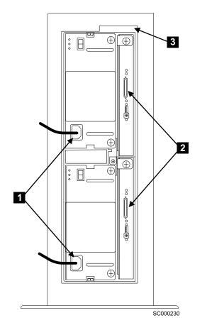
Figure 8. Power cables and SCSI connectors (2104 Model TS4)
