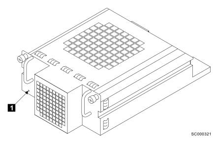
Figure 26. Fan assembly
