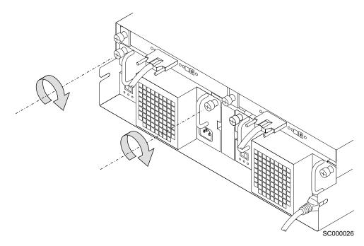
Figure 56. Tightening the screws on a fan-and-power-supply assembly
