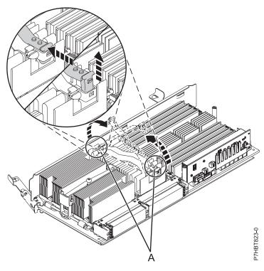
Figure 11. Unlocking the processor voltage regulator module arms
