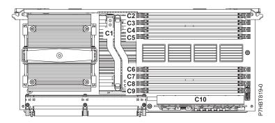
Figure 10. Processor voltage regulator module location (C1)
