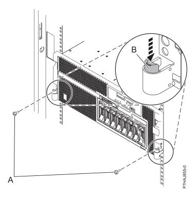
Figure 20. Releasing the rack latches
