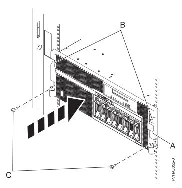
Figure 22. Replacing the thumbscrews
