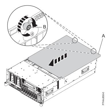
Figure 19. Installing the service access cover
