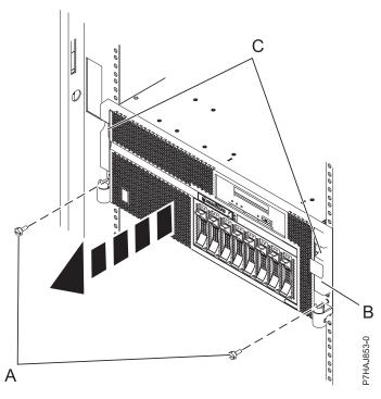
Figure 16. Removing the front cover
