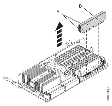
Figure 6. Removing the memory voltage regulator module
