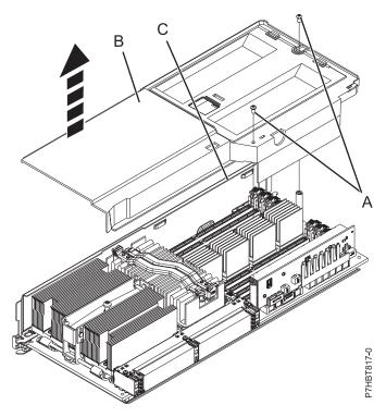
11. Locate the memory voltage regulator module to be removed from the system processor assembly. Figure 5 shows the memory voltage regulator **(C10)** in relation to the location on the system processor assembly.
