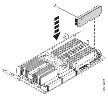
Figure 7. Memory voltage regulator module (A) shown above the voltage regulator connectors on the system processor assembly
