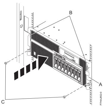
Figure 17. Installing the front cover
