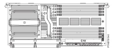
Figure 3. Memory voltage regulator module, location C10.
