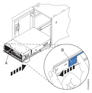
Figure 21. Releasing the rail safety latches
