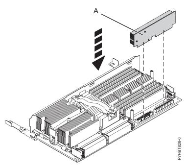
Figure 8. Installing the memory voltage regulator module
