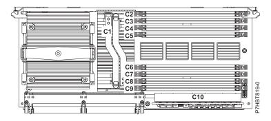
Figure 5. Memory voltage regulator module location (C10)
