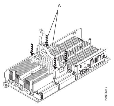
d. Using one finger on each hand, apply pressure downward on both processor voltage regulator arms at the same time, to move to the close position. Press down at the end of each arm **A** until they reach the locked position.
