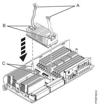
c. Use both hands to apply downward force on all four corners of the processor voltage regulator module, as shown by the arrows. When the arms are in the half open position, the voltage regulator module is in place.
