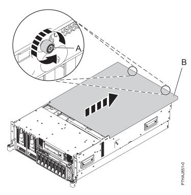
Figure 18. Removing the service access cover
