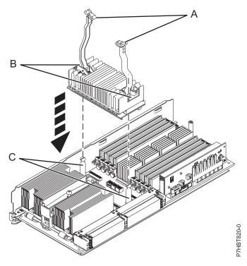
Figure 13. Processor voltage regulator module shown above the location in the system processor assembly
