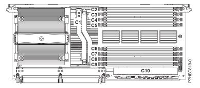
Figure 9. Processor voltage regulator module, location C1.
