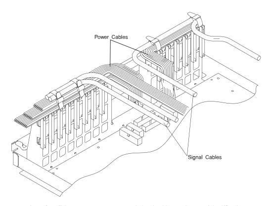
**Attention:** Take care to route power and signal cables on the top of the I/O adapter support. To keep the air-entry cutouts open in the drawer and to help prevent adapters from overheating, retain the cables with unlocking wire ties as shown.
