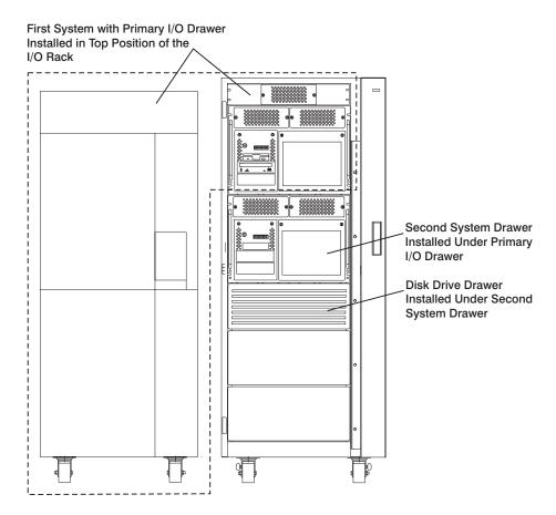
**Note:** Ensure that the cables from the I/O drawer are tied to the sides of the rack to enable servicing of the system installed under the I/O drawers.
