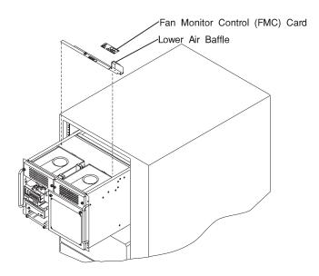
Remove the screws from the fan monitor control card and remove the card from the lower air baffle.
