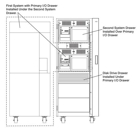
**Note:** Ensure that the cables from the upper drawers are tied to the sides of the rack to enable servicing of the lower drawers.
