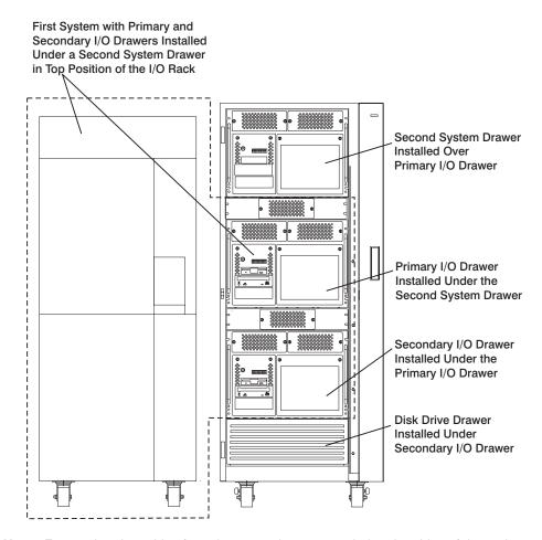
**Note:** Ensure that the cables from the upper drawers are tied to the sides of the rack to enable servicing of the lower drawers.
