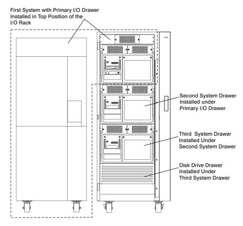
**Note:** Ensure that the cables from the I/O drawer are tied to the sides of the rack to enable servicing of the system drawers installed under the I/O drawers.
