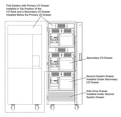
**Note:** Ensure that the cables from the I/O drawers are tied to the sides of the rack to enable servicing of the system drawer installed under the secondary I/O drawers.
