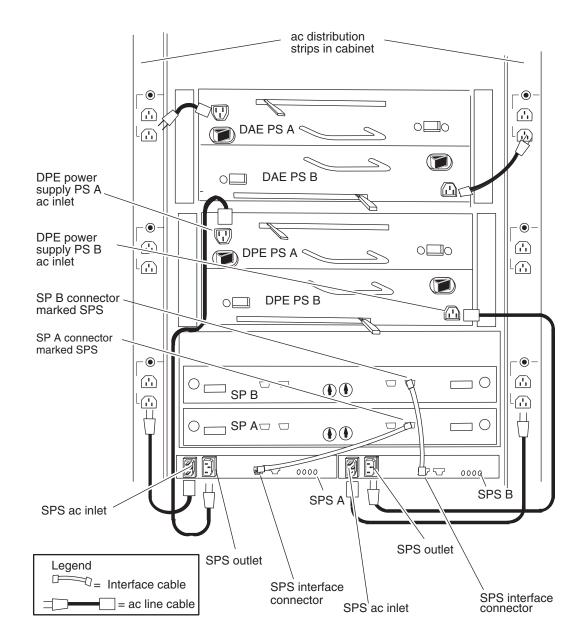
Cabling diagram for rackmount installation, showing Model 4400 or 5600 SPs (with the SPS port on the right) from back
