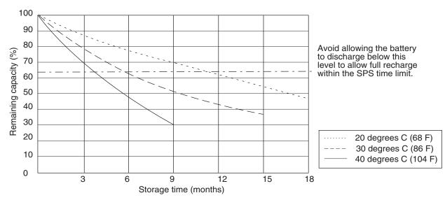
Typical SPS self-discharge levels at different storage temperatures
