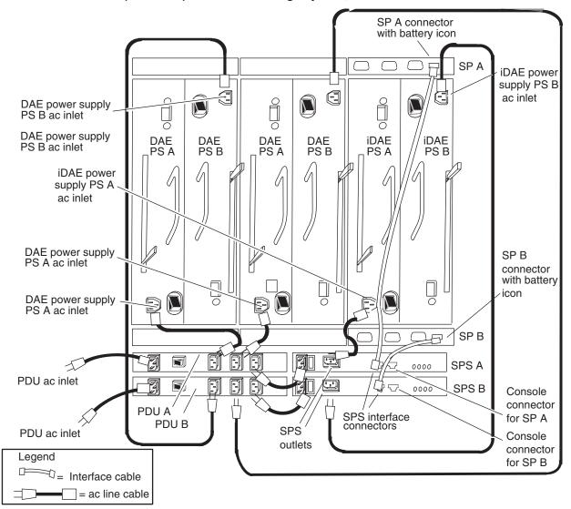
iDAE cabling diagram for deskside storage system, showing Model 4200 SPs (iDAE SPs) in a 30-slot storage system, from back
