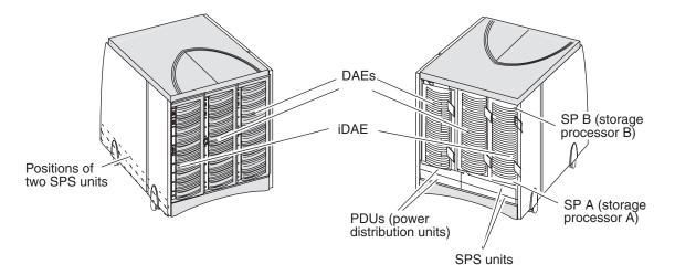
On a power failure, an SPS provides backup power until the SP has flushed its write cache data to the iDAE/DPE disks. Then the SP shuts the SPS power off. If the cache flush has not completed within 90 seconds — more than enough time to flush a full cache — or if the SP has failed, then the SPS shuts itself down to prevent deep discharge. If there is no ac inlet power and the SPS is shut down, all status lights will be off.
