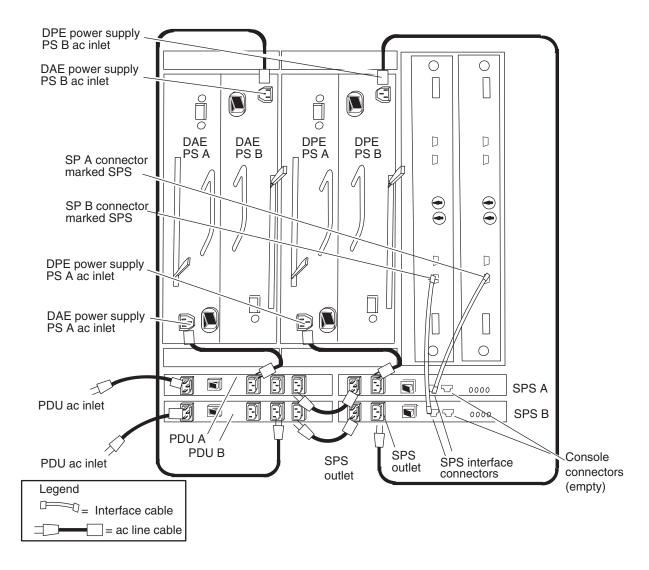
Cabling diagram for deskside storage system, showing Model 5400 SPs (with the SPS port at the bottom) from back
