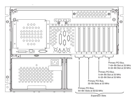
(System Unit Rear View with Numbered Slots)
