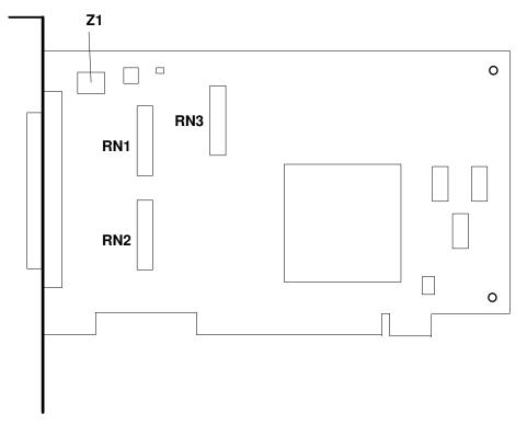
RN1, RN2 and RN3: differential terminator chips.
