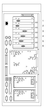
System Unit Rear View with 4-Slot PCI Riser Numbered Slots
