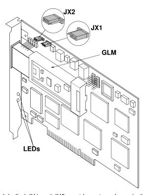
Jumpers labelled JX1 and JX2 must be set as shown in the figure above.
