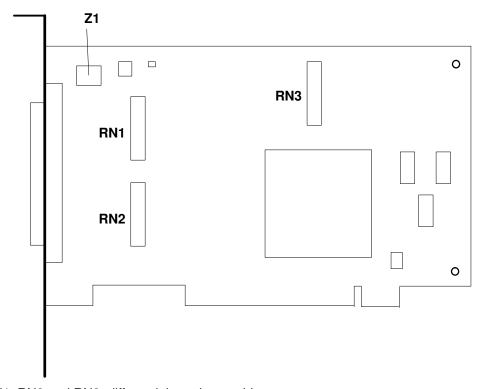
RN1, RN2 and RN3: differential terminator chips.
