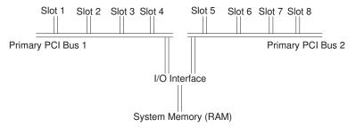
This design improves I/O performance over the secondary bus method because the I/O interface has created multiple parallel paths into the system memory.
