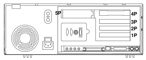
(System Unit rear view with numbered slots)
