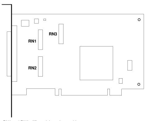
RN1, RN2 and RN3: differential terminator chips.
