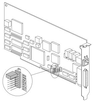
The I/O address is set by positioning a jumper on the pins corresponding to the address (see figure above). The I/O address selected in the figure is 384 the adapter's default position.
