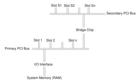
Because the slots on the secondary PCI bus must pass through the bridge chip, certain adapters on a secondary PCI bus may experience lower performance.
