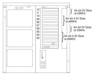
(System Unit Rear View with Numbered Slots)
