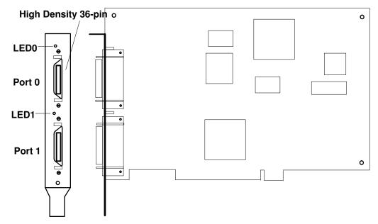
**Note:** For adapter label 8-L, the port denomination is slightly different. Port 0 is called Port 1 and Port 1 in the figure above is called Port 2.
