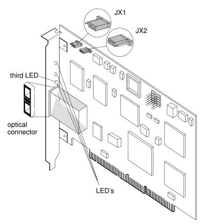
Jumpers labelled JX1 and JX2 must be set as shown in the figure above.
