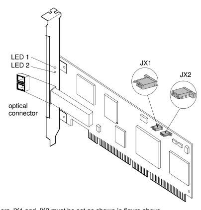
The jumpers JX1 and JX2 must be set as shown in figure above.
