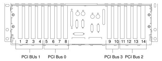
(I/O Drawer Rear View with 14 Slots and 4 PCI Buses)
