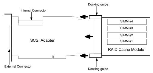
Different SIMM sizes may be mixed, however, the SIMMs must be installed so that socket #1 always contain the largest SIMM, and so on, until socket #4 which must contain the smallest SIMM.
