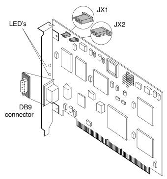
Jumpers labelled JX1 and JX2 must be set as shown in the figure above.
