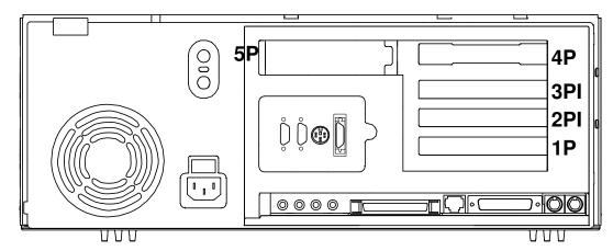
(System Unit rear view with numbered slots)
