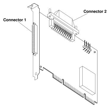
Connector 1 and connector 2 are physically connected within the adapter. There is no internal termination. You can plug either an internal cable and disks, or an external cable and disks but not at the same time.
