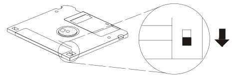
To allow writing onto a diskette, slide the write-protect tab to cover the protect slot, as shown in the following illustration.
