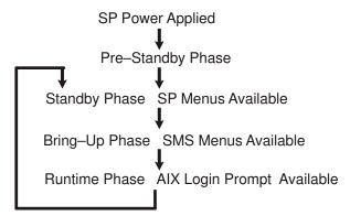
This phase is entered when the server is connected to a power source. The server may or may not be fully powered on. This phase is exited when the Power-On Self-Tests (POSTs) and configurations tasks are completed.
