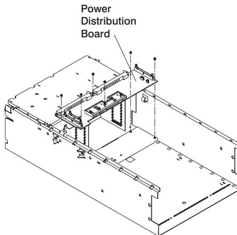
14. Remove the power distribution board.
