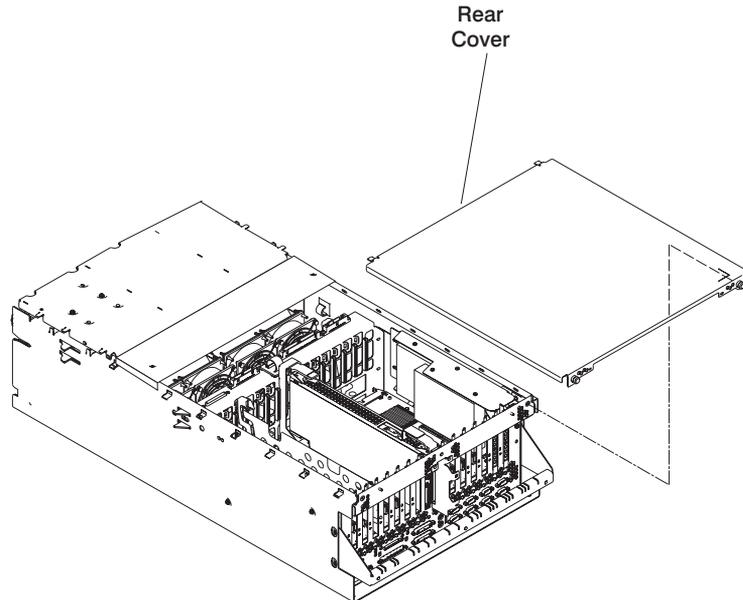
4. Disconnect and label all cables from the rear of the assembly.
