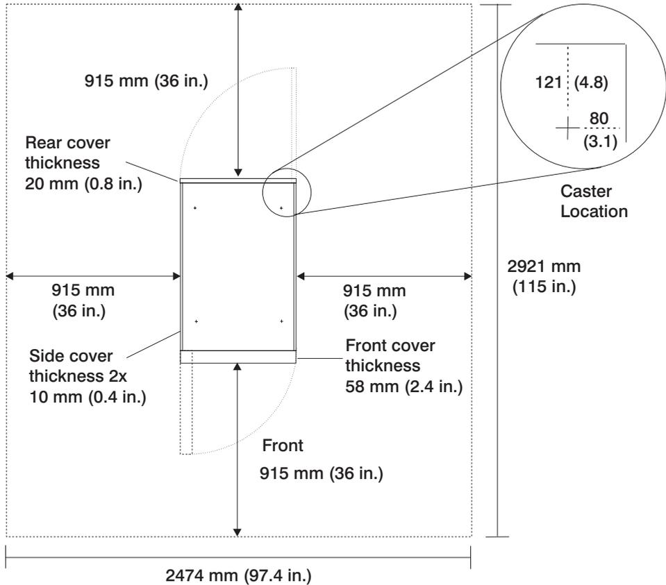
**Note:** Rack units are large and heavy and are not easily moved. Because maintenance activities require access at both the front and back, allow for extra room. The footprint shows the radius of the swinging doors on the I/O rack. The figure shows the minimum space required.
