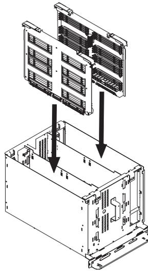
5. Locate the memory module connectors and determine which memory modules you want to remove. Refer to “Memory Riser Card and Memory DIMM Locations” on page 20 for memory module locations.
