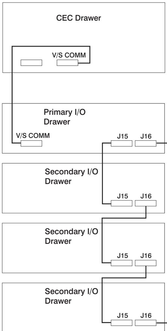
**Note:** The V/S COMM cable incorporates SPCN wiring.
