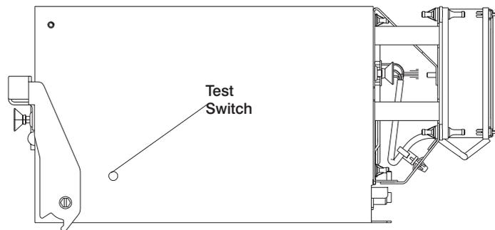
3. Use a pencil to press the test switch on the side of the power supply.
