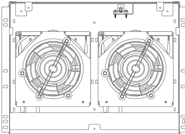
1. Loosen the two thumbscrews that attach the front bezel to the drawer.
