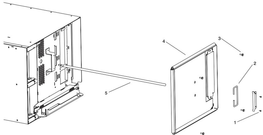
5. Remove the two card-cage retaining screws in the back of the CEC drawer.
