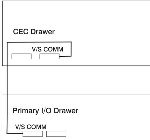
**Note:** The V/S COMM cable incorporates SPCN wiring.
