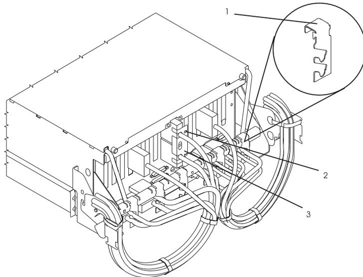
**CEC Drawer Cables:** Arrange the CEC drawer cables in the CEC drawer cable bracket **(3)**, part number 11K0249, and fasten the bracket to the back of the CEC drawer. (Fasteners **(1)** push in to lock and pull out to unlock.)
