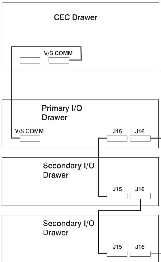
**Note:** The V/S COMM cable incorporates SPCN wiring.
