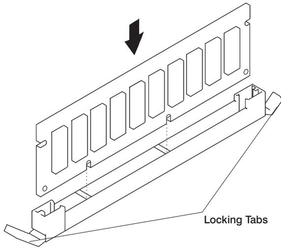
4. Secure the memory module with the locking tabs located at each end of the connector.
