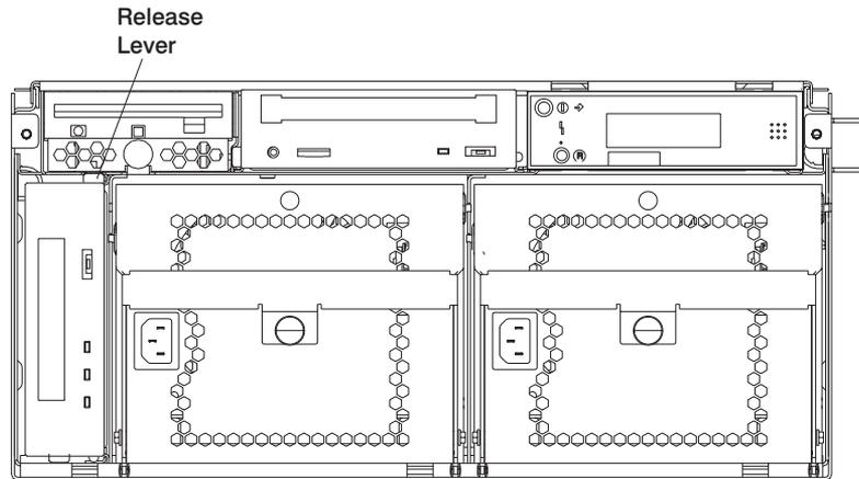
6. Disconnect the cables from the tape drive.
