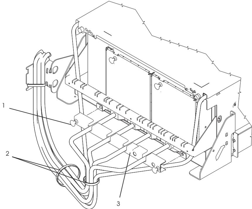
**Securing Drawer Cables:** Route the cables over the cable guides (2) and secure the cables with Velcro strips (1), part number 07H6855 or 51H9502. Leave a loop large enough so that the drawer can be pulled out the back.
