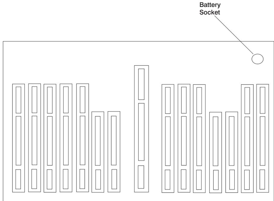
4. Remove any adapters or DASD in slots 13 and 14 to gain access to the battery.
