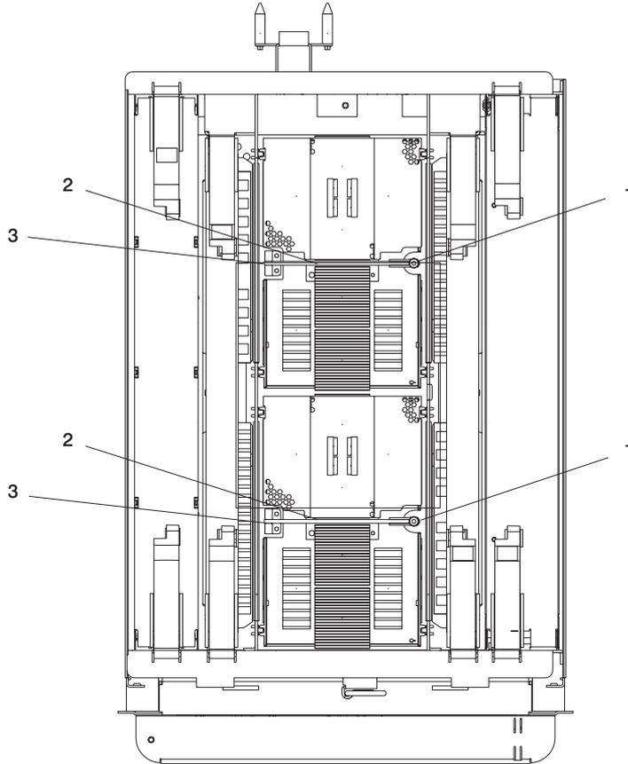
7. Locate the spring screws **(1)** attached to the processor card you want to remove. Using a 3/8" hex driver, turn the spring screw counterclockwise to loosen and remove the screw. Do not drop the screw into the CEC card-cage.
