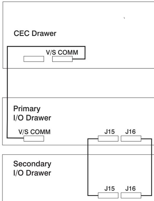
**Note:** The V/S COMM cable incorporates SPCN wiring.
