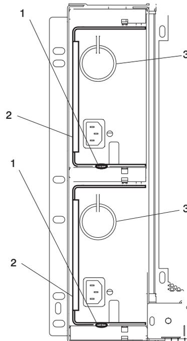
1. Carefully remove the end of the ac cord on the CEC power supply you want to replace. *Do not* remove both ac cords, as power will be lost to the CEC, forcing the system to power off.
