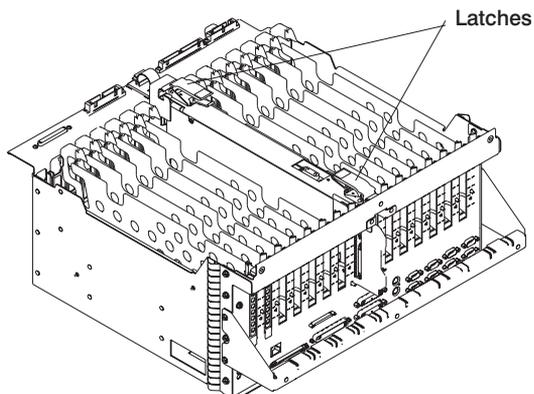
5. Remove the screw and remove the retainer bracket from the rear release latch.
