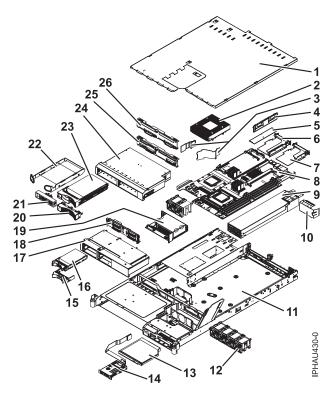
Figure 3. Models 7310-CR4 and 7042-CR4 parts illustration
