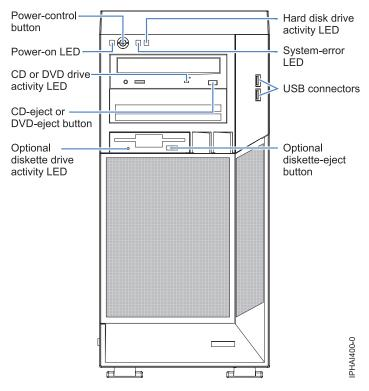
Figure 2. Model 7042-C06 and Model 7042-C07(Front view)
