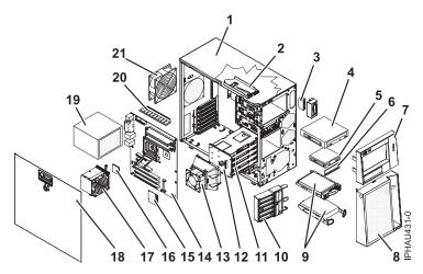
Figure 5. Model 7042-C07 parts illustration
