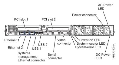
Figure 6. Back view of a typical rack-mounted HMC
