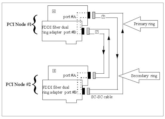
Figure 49. INTCF05: FDDI Interconnect for 2 Nodes. Case: EPC1200, EPC1200A and/or EPC400 Nodes.
