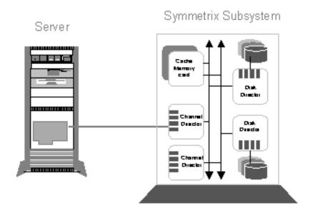
Figure 122. Point- to-point connection of an EMC<sup>2</sup> Symmetrix subsystem
