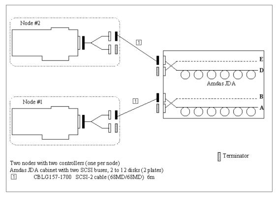
Figure 114. JDACF03: 2 nodes + 2 controllers (1 per node), 2 SCSI buses, 2 plates.
