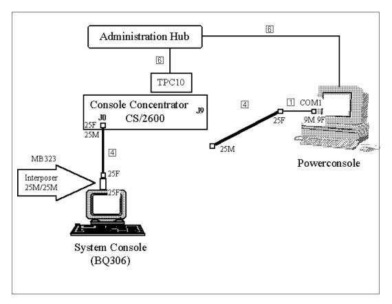
Figure 28. PowerConsole to Console Concentrator and Administration Hub
