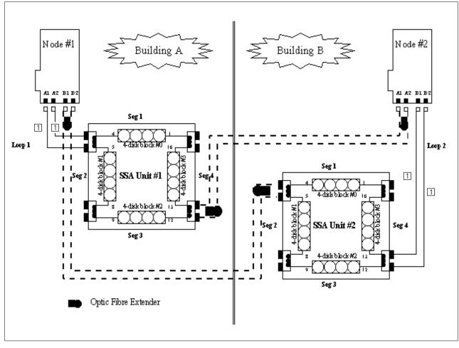
Figure 72. Cabling schema with Flbre Optical Extenders (1 or 2 nodes, 1 SSA cabinet on each side).
