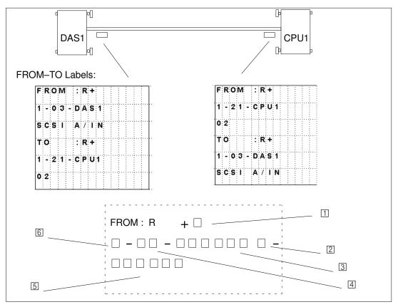
Figure 139. Cable Identification Codes on Labels.
