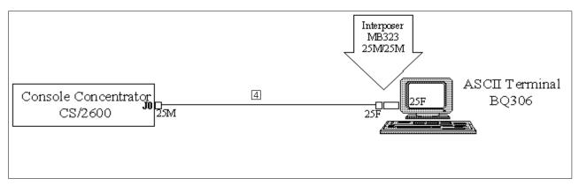
Figure 11. Cabling of the System Console to the Console Concentrator
