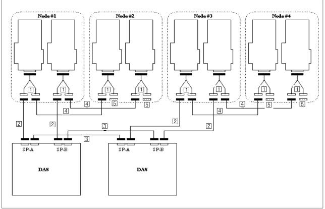
Figure 86. DASCF12: Dual SP / Dual SCSI with up to 4 nodes - Daisy chained DAS (2).
