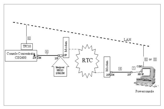
Figure 29. PowerConsole with Remote Access (LAN or Modem)
