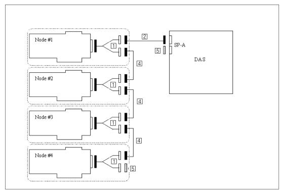
Figure 79. DASCF05: Single SP / Single SCSI with up to 4 nodes - one DAS (1). See also Figure 80.
