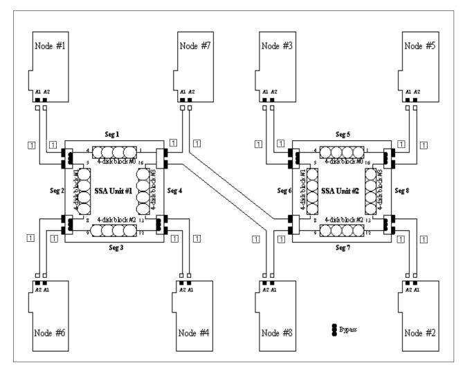
Figure 65. SSACF04: Cabling example for 8 nodes, 2 SSA cabinets and 32 disks.
