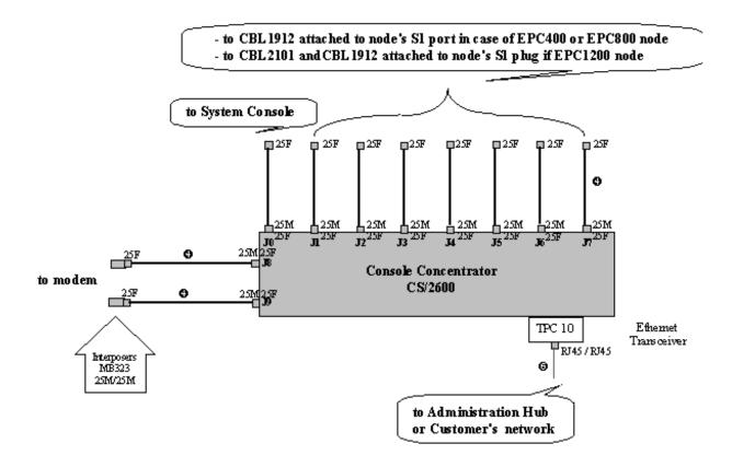
Figure 15. Console Concentrator Cabling DCKU115-2000
