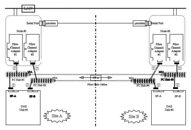
Figure 110.XLOOP02: 2 Nodes, Dual Loop, 4 Hubs, 2 DAS.
