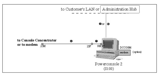
Figure 27. Escala S Series based PowerConsole Connections
