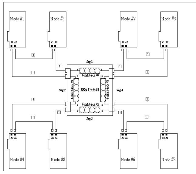
Figure 62. SSACF03: Cabling example for 8 nodes, 1 SSA cabinet and 16 disks.
