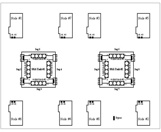
Figure 63. SSACF04: Base mounting diagram (7 to 8 nodes, 2 SSA cabinets, up to 8 segments).
