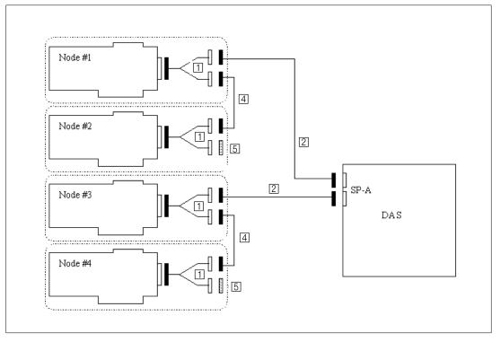
Figure 80. DASCF06: Example of Single SP / Single SCSI with up to 4 nodes – one DAS (2). See also Figure 79.
