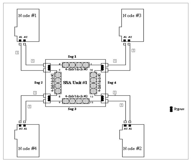
Figure 56. SSACF01: Cabling example for 4 nodes, 1 SSA cabinet and 16 disks.
