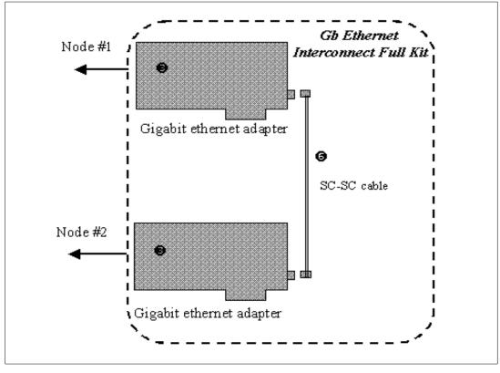
Figure 42. Gigabit Ethernet Interconnect for 2 Nodes
