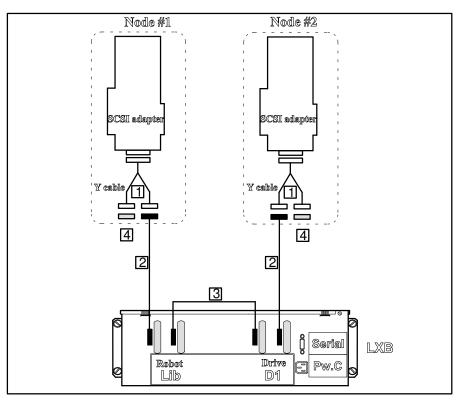
Cabling for: 2 Nodes - 1 Adapter per Node - 1 Drive
