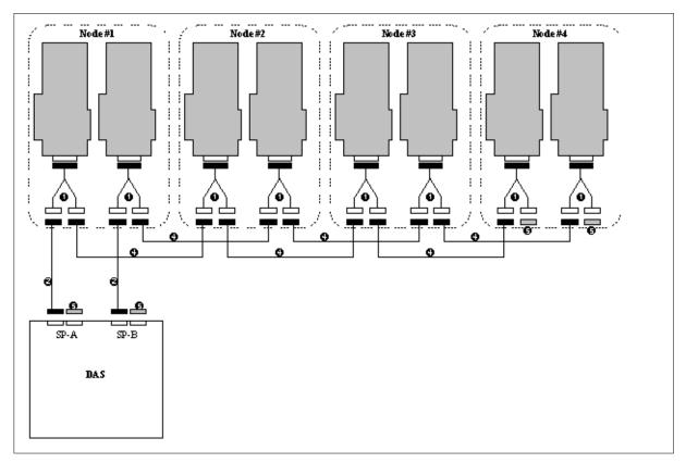
Figure 83. DASCF09: Dual SP / Dual SCSI with up to 4 nodes - 1 DAS (1).
