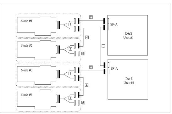
Figure 82. DASCF08: Single SP / Single SCSI with up to 4 nodes - Daisy chained DAS (2).
