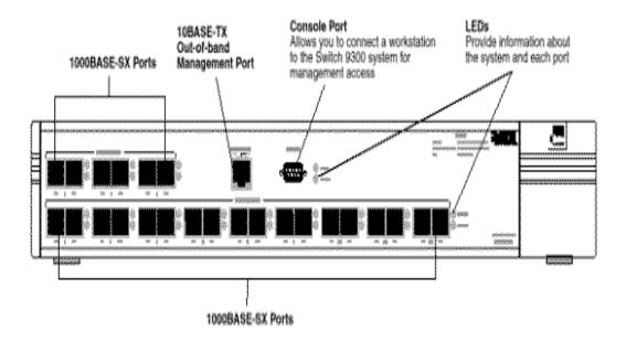
Figure 40. Switch 9300 - Front View
