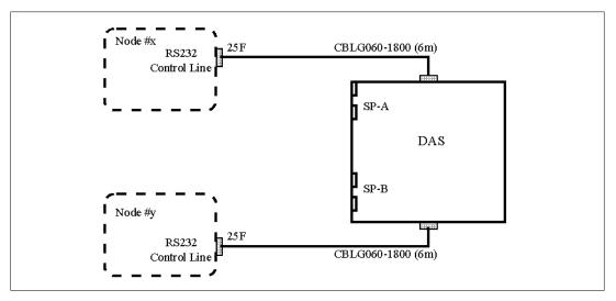
Figure 88. Cabling for Configuration & Management, 1 DAS, 2 SP.
