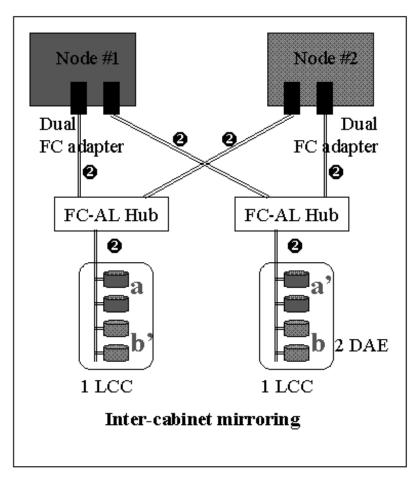
Figure 103.SLOOP04: Two Loops, 2 Nodes, 2 DAEs (1 LCC).
