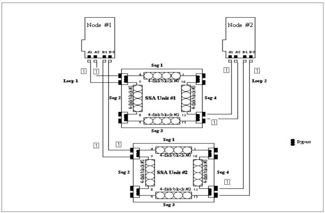
Figure 71. SSACF01 Configuration with two loops (1 or 2 nodes, 1 SSA cabinet on each side).
