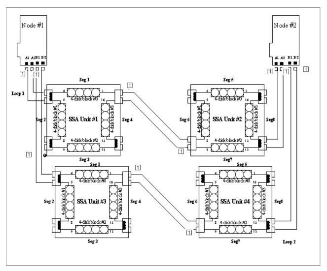
Figure 73. SSACF02 Configuration with two loops (1, 2 or 3 nodes, 2 SSA cabinets on each side).
