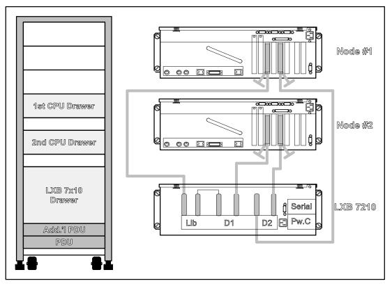
Figure 127. Overall Diagram – EPC400 with 2 nodes sharing an LXB.
