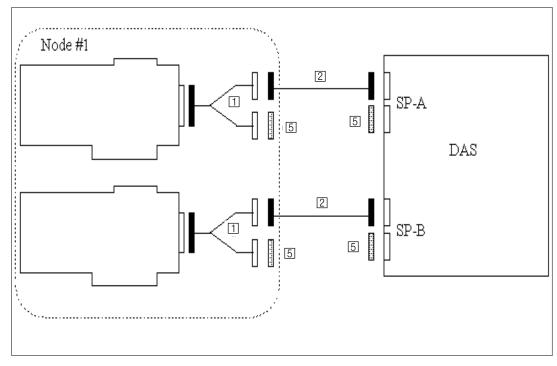
Figure 77. DASCF03: Dual SP / Dual SCSI with 1 node - 1 DAS.
