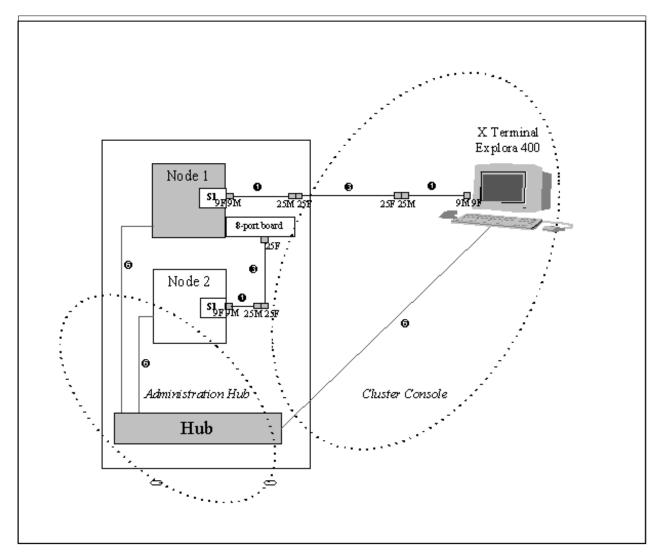
Figure 20. PWCCF02: Temporary Replacement of Cluster Console with System Console
