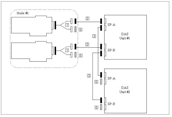
Figure 78. DASCF04: Dual SP / Dual SCSI with 1 node - Daisy chained DAS.
