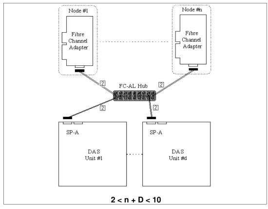
Figure 102.SLOOP03: Single Loop, 1 Hub, N Nodes, D DAS (1 SP).
