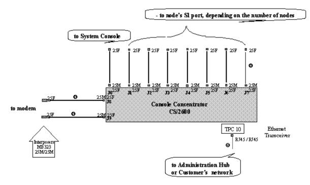
Figure 16. Console Concentrator Cabling DCKU119–2000
