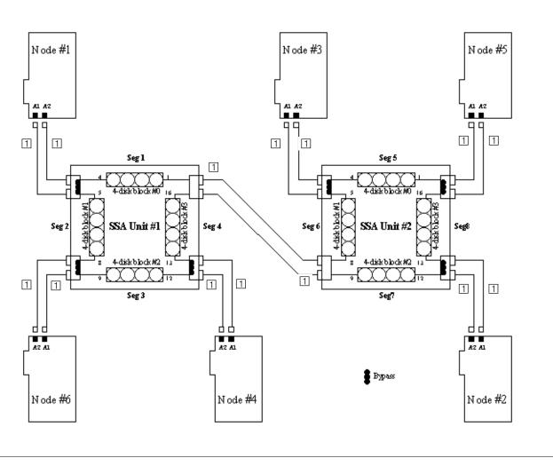
Figure 59. SSACF02: Cabling example for 6 nodes, 2 SSA cabinets and 32 disks. At least 8 disk drives are mandatory.
