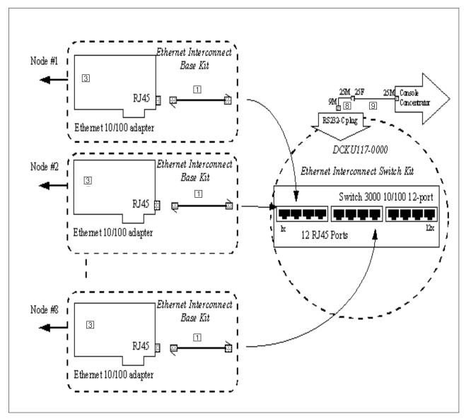
Figure 36. INTCF10: Ethernet Switch Single Interconnect for 3 to 8 Nodes with Single Adapter Per Node
