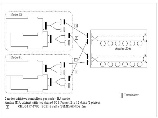
Figure 120. JDACF09: 2 nodes + 2 controllers per node - HA mode, 2 shared SCSI buses, 2 plates.
