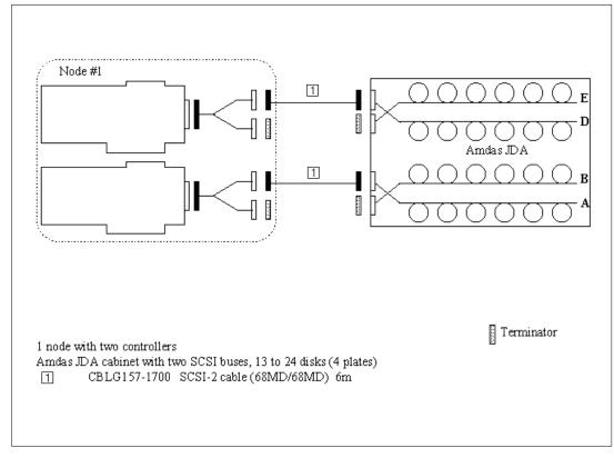
Figure 117. JDACF06: 1 node + 2 controllers, 2 SCSI buses, 4 plates.
