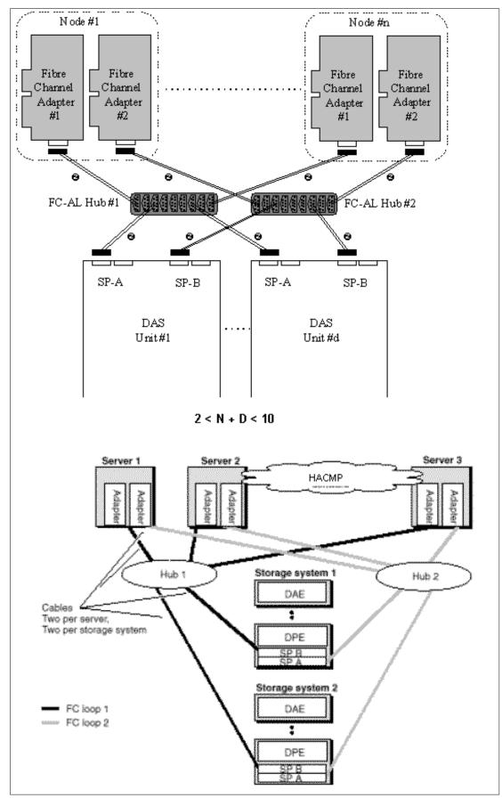
Figure 107.DLOOP03: Dual Loop, Two Hubs, N Nodes, D DAS with 2 SPs.
