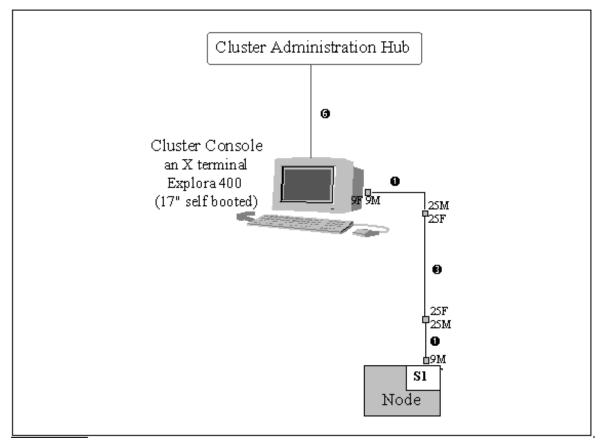
Figure 19. Cluster Console with Connection to Node's S1 Plug
