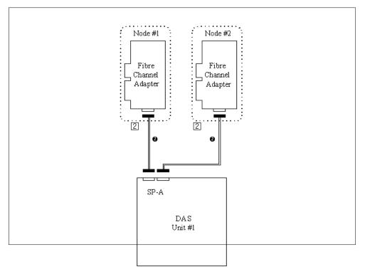
Figure 101.SLOOP02: Single Loop, 2 Nodes, 1 DAS (1 SP).
