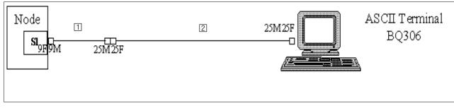
Figure 10. Cabling of the System Console to a Node's S1 Plug
