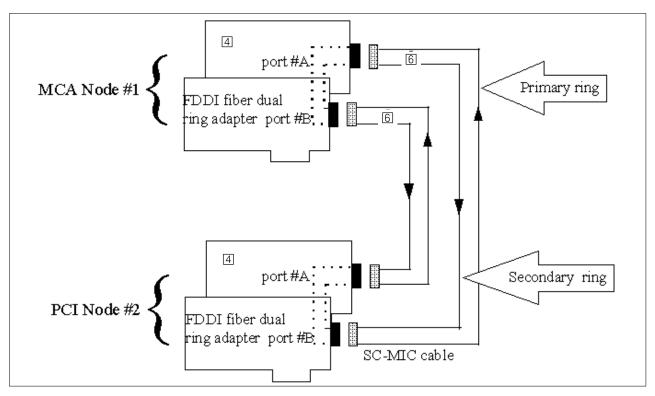
Figure 50. INTCF05: FDDI Interconnect for 2 Nodes. Mixed Case: (MCA \* PCI nodes) with an EPC800 node.
