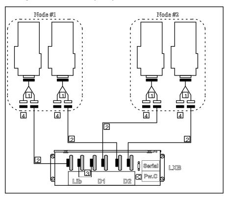
Figure 132. LIBCF03: 2 Nodes – 2 Adapters per Node – 2 Drives
