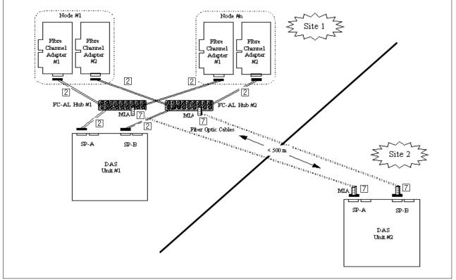
Figure 109.XLOOP02: 2 Nodes, Dual Loop, 2 Hubs, 2 DAS (one Deported).
