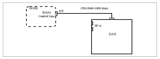
Figure 87. Cabling for Configuration & Management, 1 DAS, 1 SP.
