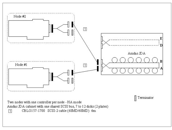
Figure 119. JDACF08: 2 nodes + 1 controller per node – HA mode , 1 shared SCSI bus, 2 plates.
