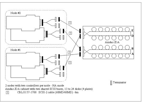
Figure 121. JDACF10: 2 nodes + 2 controllers per node – HA mode, 2 shared SCSI buses, 4 plates.
