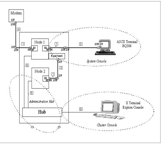
Figure 135. Remote maintenance: Modem on a Node's S2 plug without Console Concentrator.
