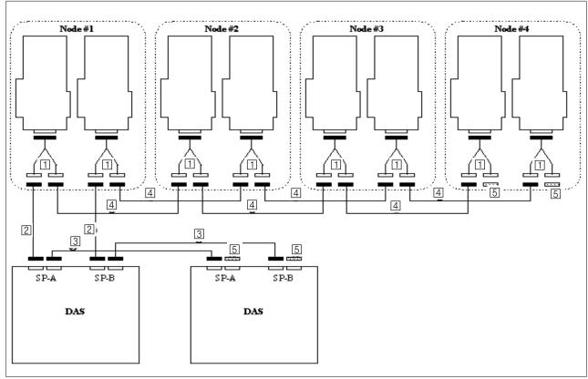
Figure 85. DASCF11: Dual SP / Dual SCSI with up to 4 nodes - Daisy chained DAS (1).
