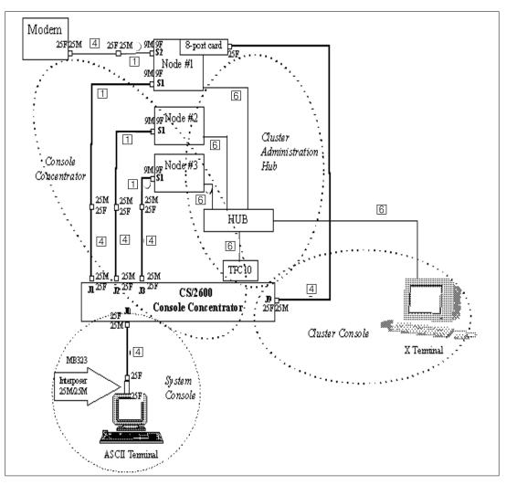
Figure 136. RMCF03: Remote maintenance: Modem on a Node's S2 plug w/ Console Concentrator
