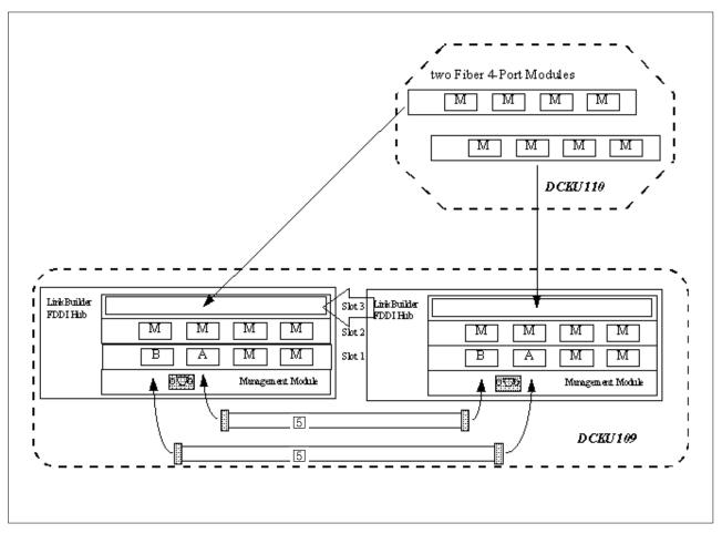
Figure 51. Components of FDDI Interconnect with Hub (Dual Homing)
