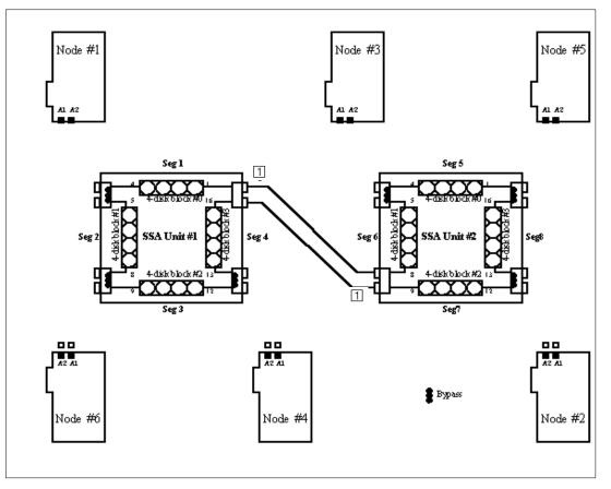
Figure 57. SSACF02: Base mounting diagram (1 to 6 nodes, two SSA cabinets, 1 to 8 segments).
