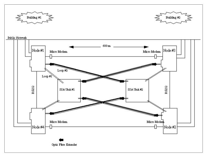
Figure 69. Optic Fibre Extender: Global diagram (1 pair of 2 nodes, 1 cabinet).
