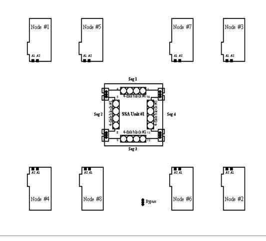
Figure 60. SSACF03: Base mounting diagram (5 to 8 nodes, 1 SSA cabinet, 1 to 4 segments).
