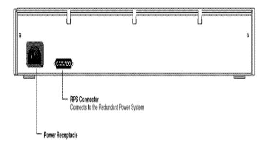
Figure 41. Switch 9300 - Rear View
