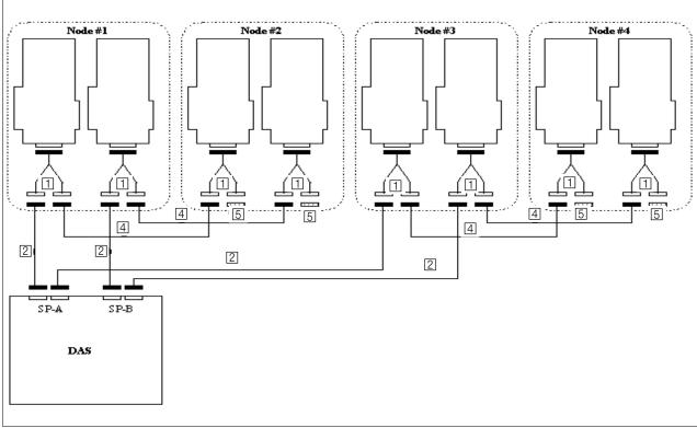
Figure 84. DASCF10: Dual SP / Dual SCSI with up to 4 nodes - 1 DAS (2).
