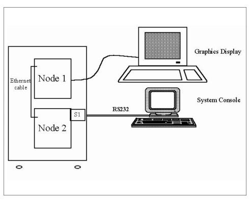
Figure 8. PWCCF08: 2-node EPC - (1 System Console, 1 Graphic Display).
