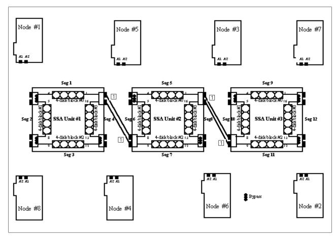
Figure 66. SSACF05: Base mounting diagram (1 to 8 nodes, 3 SSA cabinets, up to 12 segments).
