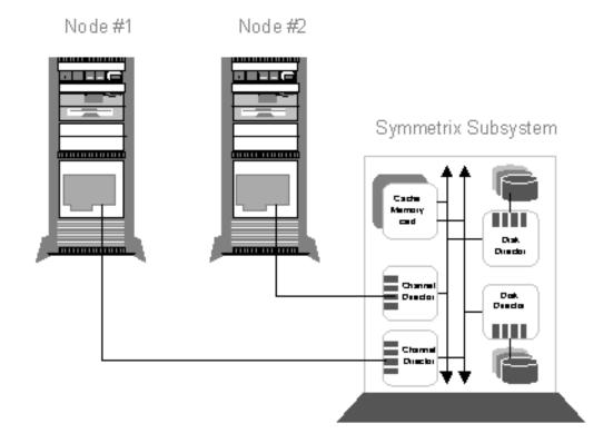
Figure 124. Base configuration of an EMC<sup>2</sup> Symmetrix subsystem with HACMP
