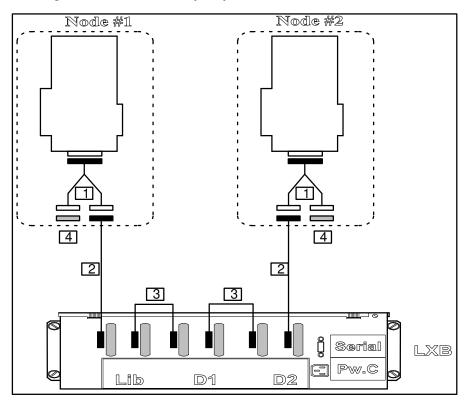
Figure 131. LIBCF02: 2 Nodes - 1 Adapter per Node - 2 Drives
