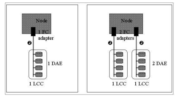
Figure 99.SLOOP00: Single Loop, 1 Node, 1 or 2 DAE.
