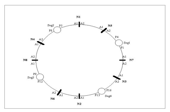
Figure 61. SSACF03: Loop diagram: 5 to 8 nodes, 1 SSA cabinet, 1 to 4 segments.
