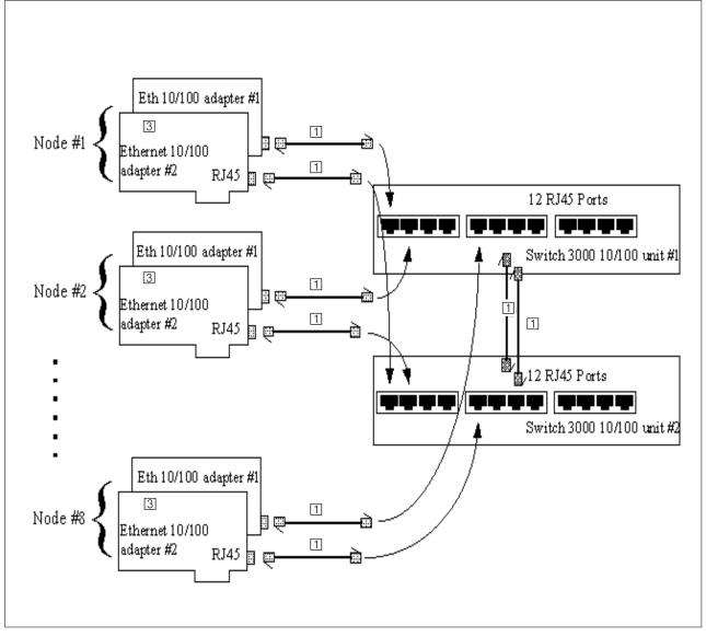
Figure 38. Redundant Fast Ethernet Interconnect for 3 to 8 Nodes
