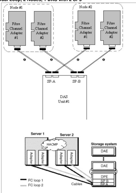
Figure 106.DLOOP02: Dual Loop, 2 Nodes, 1 DAS with 2 SPs.
