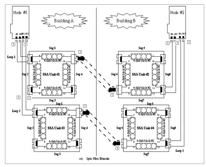
Figure 74. Cabling diagram with Flbre Optical Extenders (1, 2 or 3 nodes, 2 SSA cabinets on each side).
