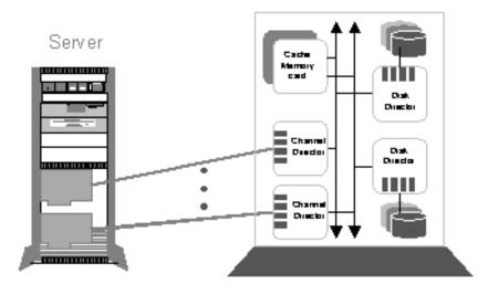
Figure 123. Multiple connection of an EMC<sup>2</sup> Symmetrix subsystem
