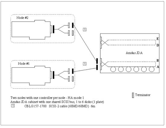
Figure 118. JDACF07: 2 nodes + 1 controller per node - HA mode , 1 shared SCSI bus, 1 plate.
