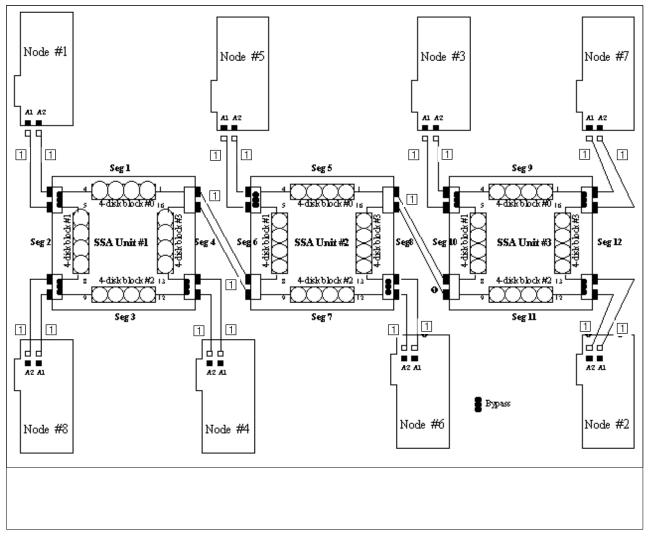
Figure 68. SSACF05: Cabling example for 8 nodes, 3 SSA cabinets and 48 disks. At least 12 disk drives are required.
