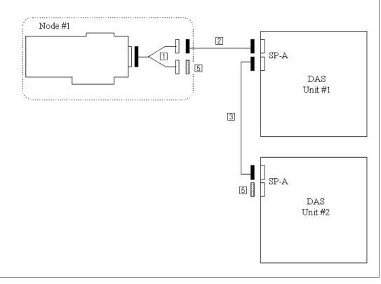
Figure 76. DASCF02: Single SP / Single SCSI with 1 node – Daisy chained DAS.
