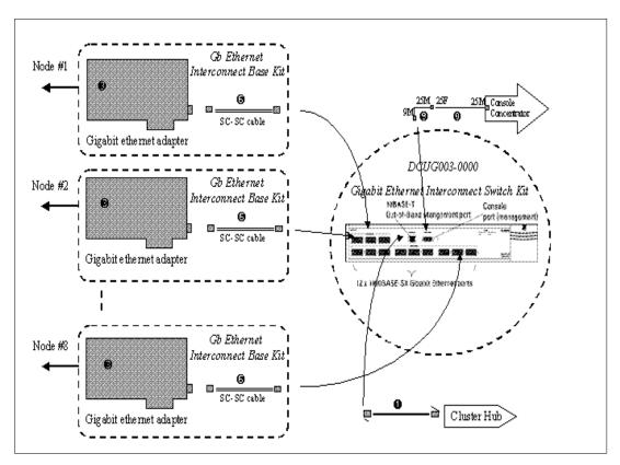
Figure 43. Gigabit Ethernet Interconnect for >2 Nodes
