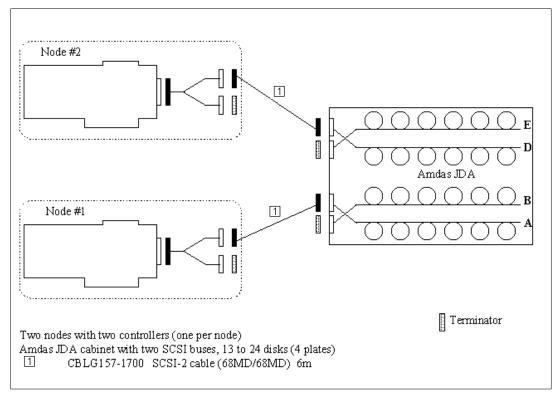
Figure 115. JDACF04: 2 nodes + 2 controllers (1 per node), 2 SCSI buses, 4 plates.
