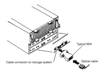
Figure 92.MIA (Media Interface Adapter) seen from the back of the storage system
