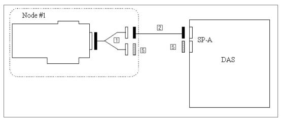
Figure 75. DASCF01: Single SP / Single SCSI with 1 node - 1 DAS.
