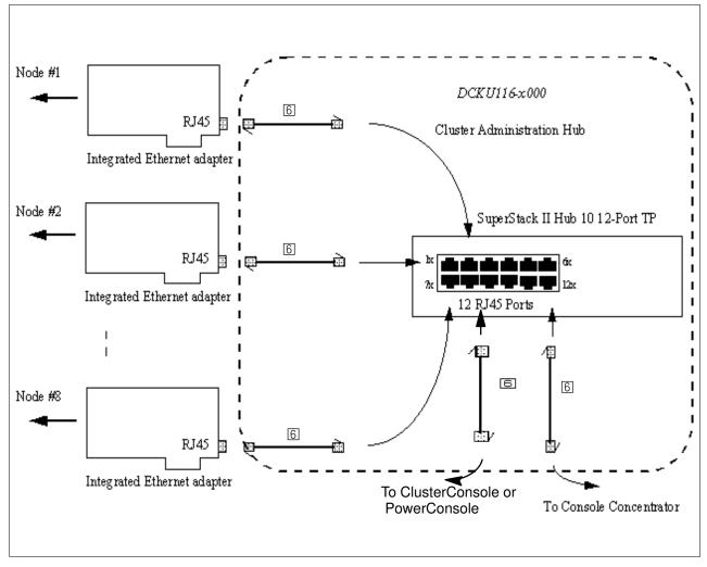
Figure 14. Cluster Administration Hub Connections to Nodes and Console
