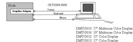
Figure 9. Cabling of the Graphics Display to a Node.
