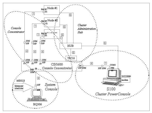
Figure 133. RMCF02:Remote maintenance: Modem on a PowerConsole (Escala S100)
