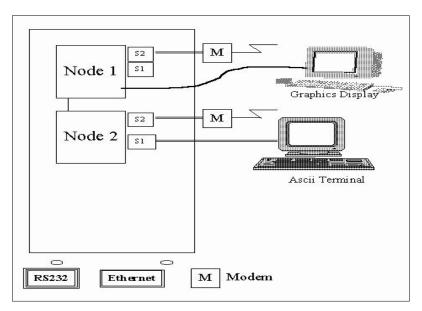
Figure 137. RMCF01: Remote maintenance: Two Modems without a Cluster Console.
