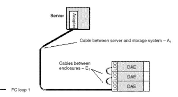
Figure 98.A chained DAE with one Link Control Card
