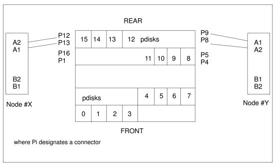
Figure 53. Example of 1 SSA cabinet and 1 adapter per node (one loop).
