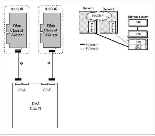
Figure 105.DLOOP04: Two Loops, 2 Nodes, 1 DAS with 2 SPs.
