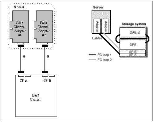
Figure 104.DLOOP01: Dual Loop, 1 Node with 2 Adapters, 1 DAS with 2 SPs.
