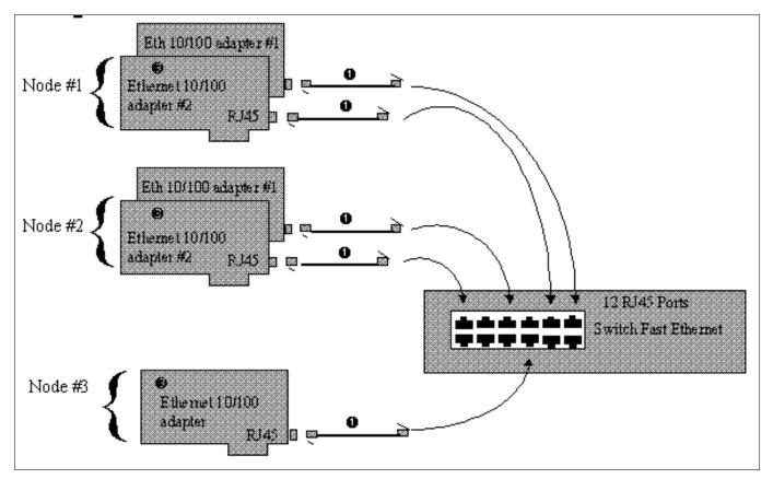
Figure 37. INTCF10: Ethernet Switch Single Interconnect for 3 to 8 Nodes with Dual Adapters Per Node
