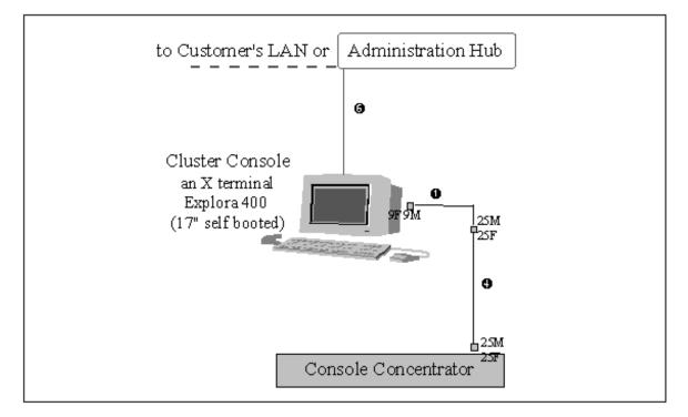
Figure 18. Cluster Console with Console Concentrator
