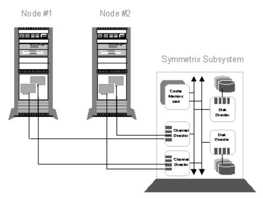
Figure 125. Configuration of an EMC<sup>2</sup> Symmetrix subsystem with Powerpath
