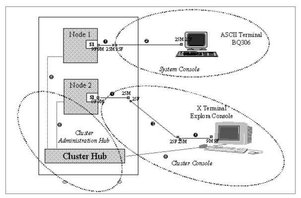
Figure 22. Alternative Cabling of Cluster Console and System Console – Both node console and common administration graphical terminal
