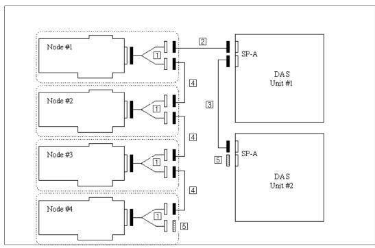
Figure 81. DASCF07: Single SP / Single SCSI with up to 4 nodes - Daisy chained DAS (1).
