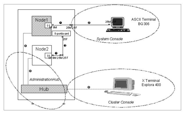
Figure 21. Alternative Cabling of Cluster Console and System Console – Common administration graphical interface
