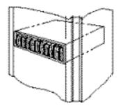
Figure 91.Disk Array Enclosure - DAE
