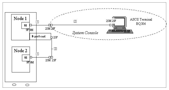
Figure 12. PWCCF01: Cabling Schema for a 2-node Powercluster
