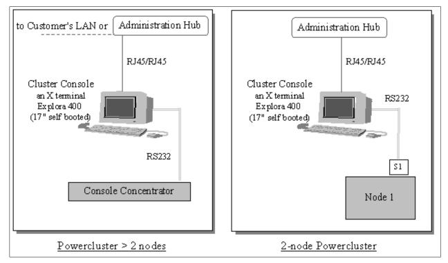
Figure 17. Cluster Console with Powercluster 2 Nodes and >2 Nodes
