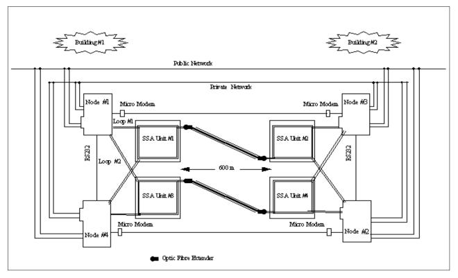
Figure 70. Optic Fibre Extender: Global diagram (1 pair of 2 nodes, 2 cabinets).
