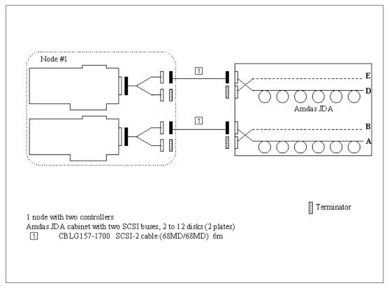
Figure 116. JDACF05: 1 node + 2 controllers, 2 SCSI buses, 2 plates.
