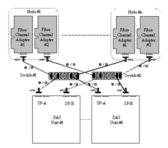
$0 < N + D \le 16$ The connectors of the switch that are black on the figure are equipped with GBICs.
