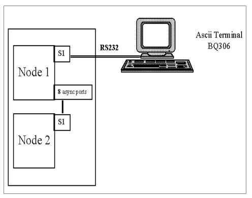
Figure 6. PWCCF01: 2-node Escala EPC - (one System Console).
