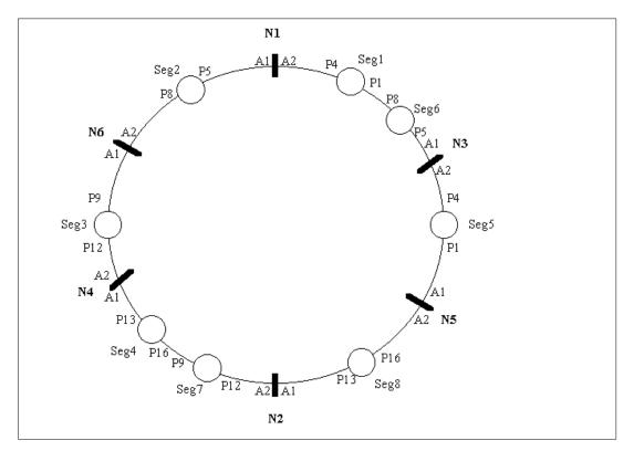
Figure 58. SSACF02: Loop diagram: 1 to 6 nodes, 2 SSA cabinets, 5 to 8 segments.
