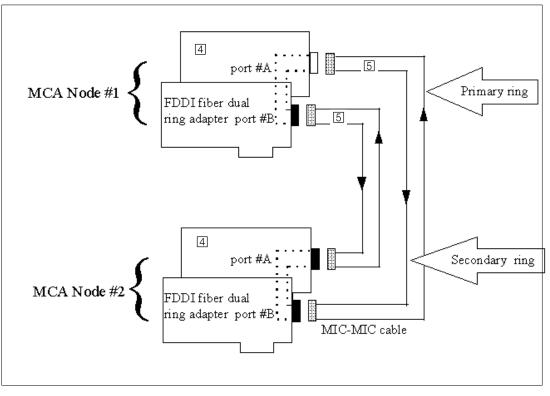
Figure 48. INTCF05: FDDI Interconnect for 2 Nodes. Case: EPC800 Nodes.
