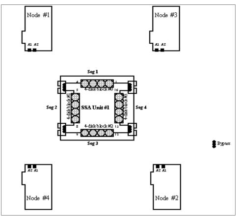
Figure 54. SSACF01: Base mounting diagram (1 to 4 nodes, 1 SSA cabinet, 1 to 4 segments).
