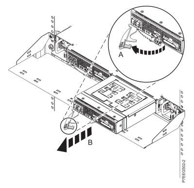
Figure 1. Removing an ERM assembly from the enclosure
