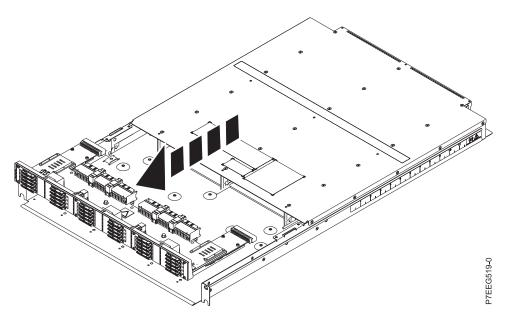
Figure 11. Removing the midplane
