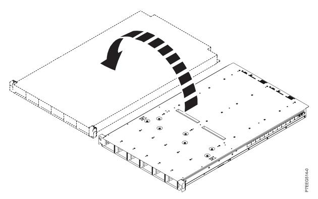
Figure 18. Turning the enclosure top side up
