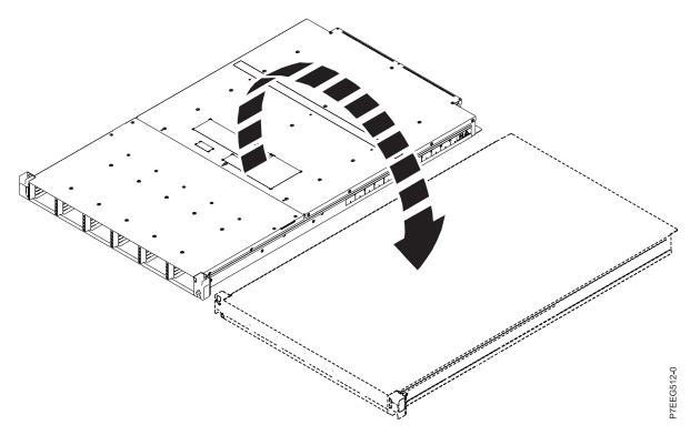
Figure 16. Turning the enclosure upside down
