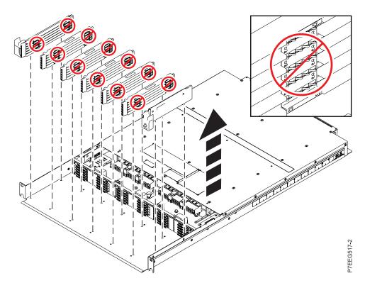
Figure 9. Removing the solid-state drive rails
