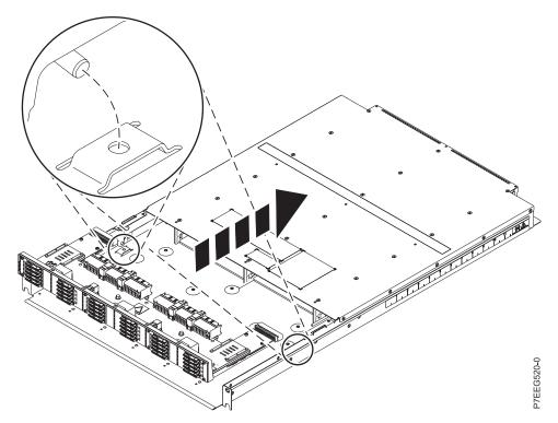
Figure 12. Installing the midplane
