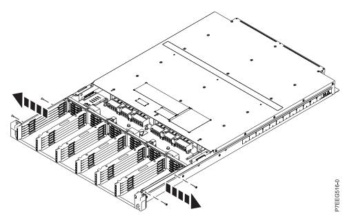
Figure 8. Removing the screws on the right and left sides of the enclosure
