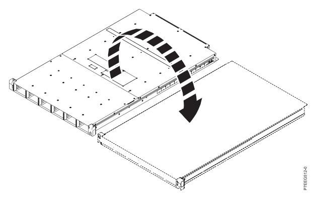
Figure 4. Turning the enclosure upside down
