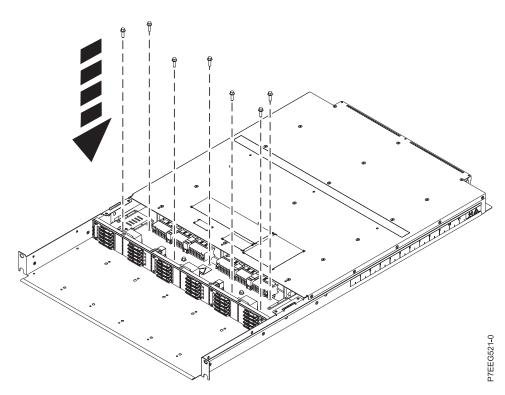
Figure 13. Installing the midplane screws
