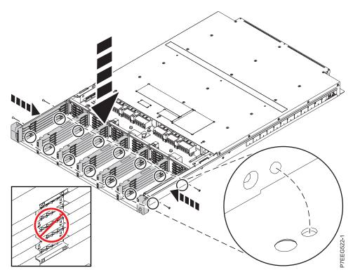
Figure 14. Installing the solid-state drive rails
