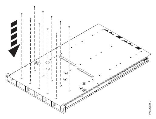
Figure 17. Installing the screws to the bottom of the enclosure
