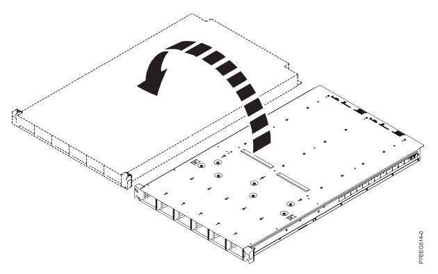
Figure 6. Turning the enclosure top side up
