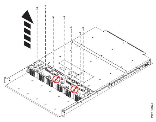
Figure 10. Removing the midplane screws
