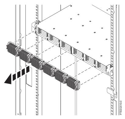
Figure 3. Removing the bezels
