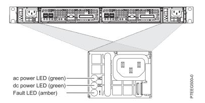
Figure 19. Rear view of power supply
