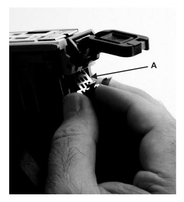
Install the metal EMC shield (A) to the top of the tailstock.
