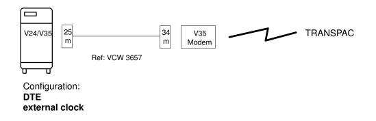
Figure 50. V24/V35 Connection to TRANSPAC Network
