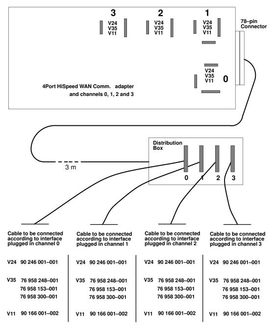
Figure 24. 4Port HiSpeed WAN Comm.: Connection of the cables on the distribution box
