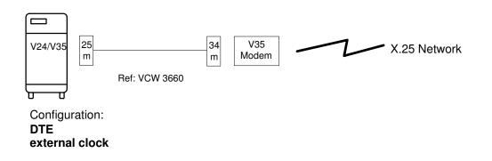
Figure 51. V24/V35 Connection to a Public Network (EIA Standard)
