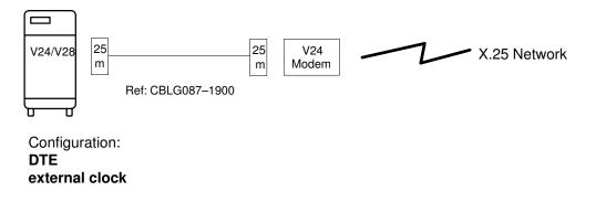
Figure 47. V24/V28 Connection to a Network
