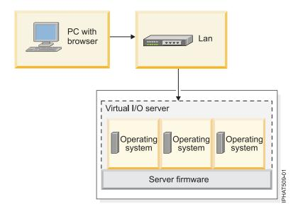
This figure illustrates an IBM Power Systems server or an IBM BladeCenter blade server with POWER® Architecture technology. The Virtual I/O Server is in its own logical partition, and the client logical partitions are managed by the Virtual I/O Server logical partition. The browser on the PC connects to the Integrated Virtualization Manager interface over a network, and you can use the Integrated Virtualization Manager to create and manage the logical partitions on the server.
