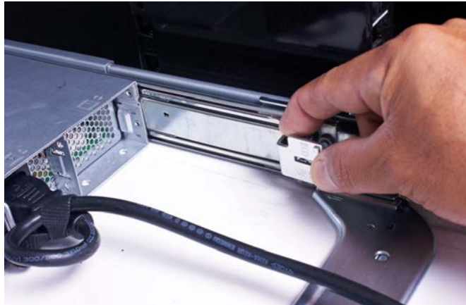
Figure 4. Attaching the inner CMA attachment bracket
