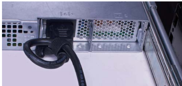
Figure 3. Routing the power cable through the strain relief on a fixed power supply
