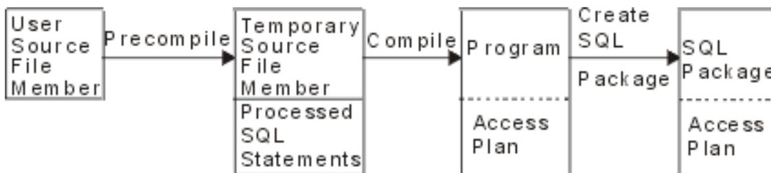
With a distributed ILE DB2 UDB for iSeries program, you must manage the original source, module objects, the resulting program or service program, and the resulting packages. An SQL package can be created for each distributed module in a distributed ILE program or service program. The following figure shows the objects and the steps that occur during the precompile and compile processes for a distributed ILE DB2 UDB for iSeries program:
