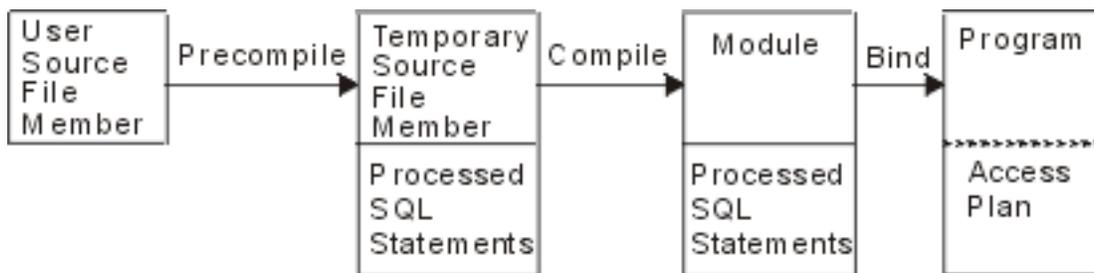
With a distributed non-ILE DB2 UDB for iSeries program, you must manage the original source, the resulting program, and the resulting package. The following figure shows the objects and the steps that occur during the precompile and compile processes for a distributed non-ILE DB2 UDB for iSeries program:
