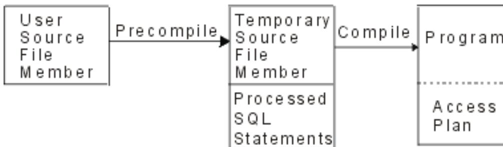
With a nondistributed ILE DB2 UDB for iSeries program, you might need to manage the original source, the modules, and the resulting program or service program. The following figure shows the objects involved and the steps that happen during the precompile and compile processes for a nondistributed ILE DB2 UDB for iSeries program when OBJTYPE(\*PGM) is specified on the precompile command:
