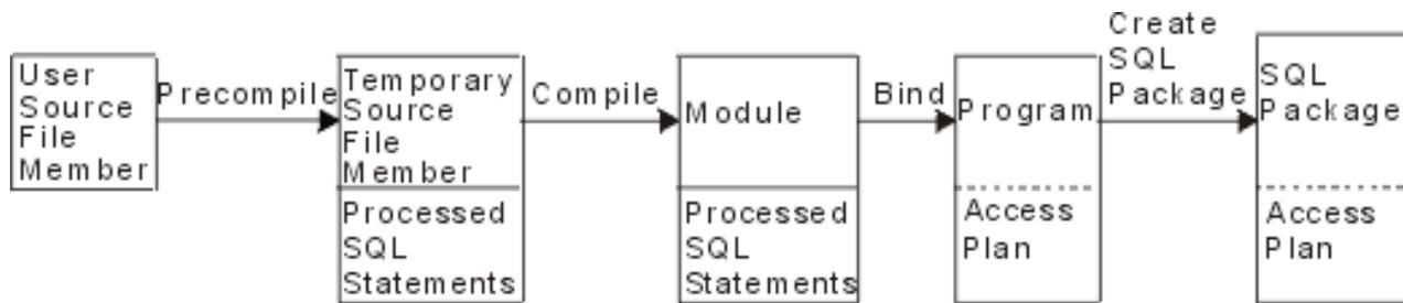
**Note:** The access plans associated with the DB2 UDB for iSeries distributed program object are not created until the program is run locally.
