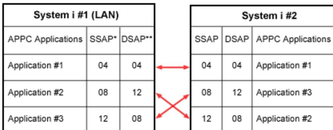
\* The LAN source service access point (SSAP) is the logical address that this system sends with any data to a remote system. This value must match the DSAP of the remote controller.
