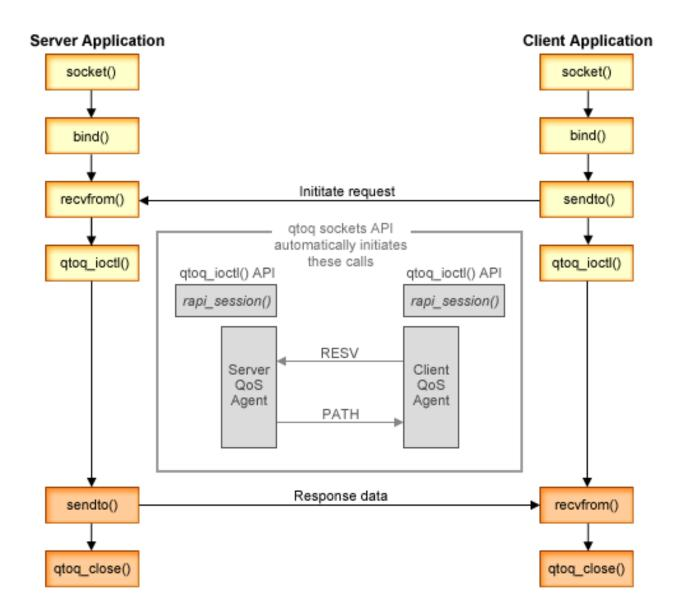
**qtoq flow of events**: The following sequence of socket calls provides a description of the figure. It also describes the relationship between the server and client application in a connectionless design. These are modifications of the basic socket APIs.
