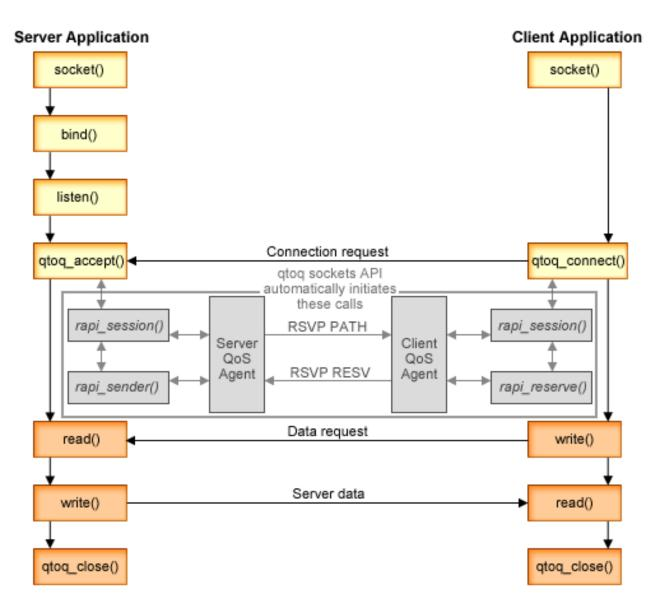
**qtoq flow of events:** The following sequence of socket calls provides a description of the figure. It also describes the relationship between the server and client application in a connection-oriented design. These are modifications of the basic socket APIs.
