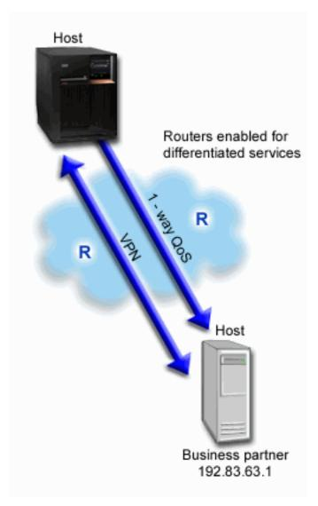
Figure 5. Host-to-host VPN connection using a QoS differentiated service policy
