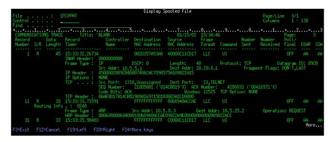
This figure shows the TCP/IP data portion of the communications trace.
