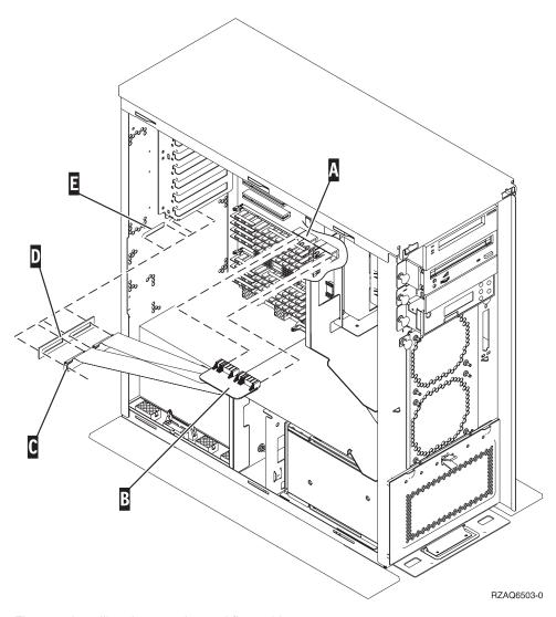
Figure 5. Installing the 7002 internal flex cable
