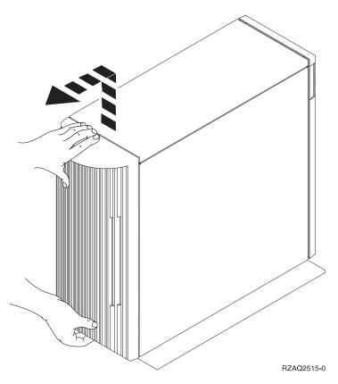
Figure 13. Removing the system unit or expansion unit back cover
