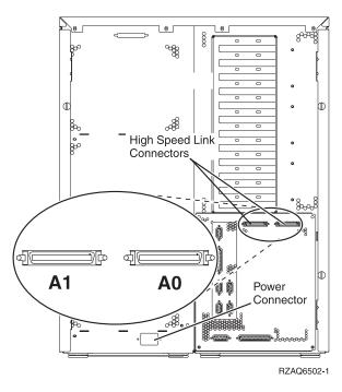
Figure 17. 820 HSL connector locations
