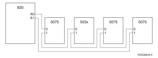
Figure 23. HSL loop with four external units
