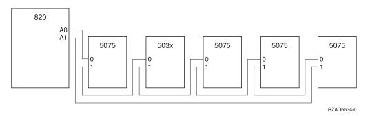
Figure 24. HSL loop with five external units
