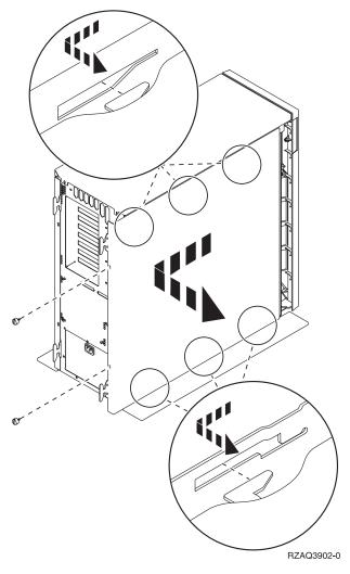
Figure 3. Remove system unit side cover
