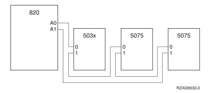
Figure 22. HSL loop with three external units
