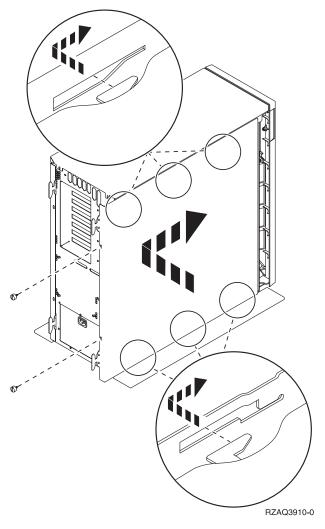
Figure 6. Install system unit side cover
