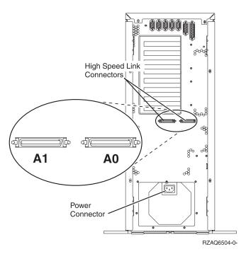
Figure 16. 270 HSL connector locations
