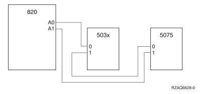
Figure 21. HSL loop with two external units
