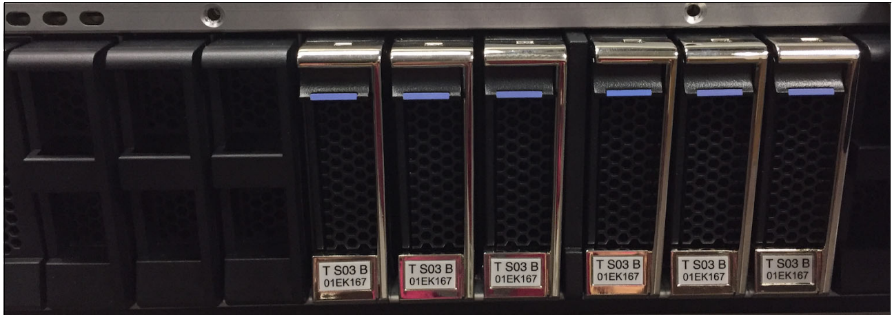
Figure 1-3 Six IBM MicroLatency modules and three flash module filler cards installed in the machine
