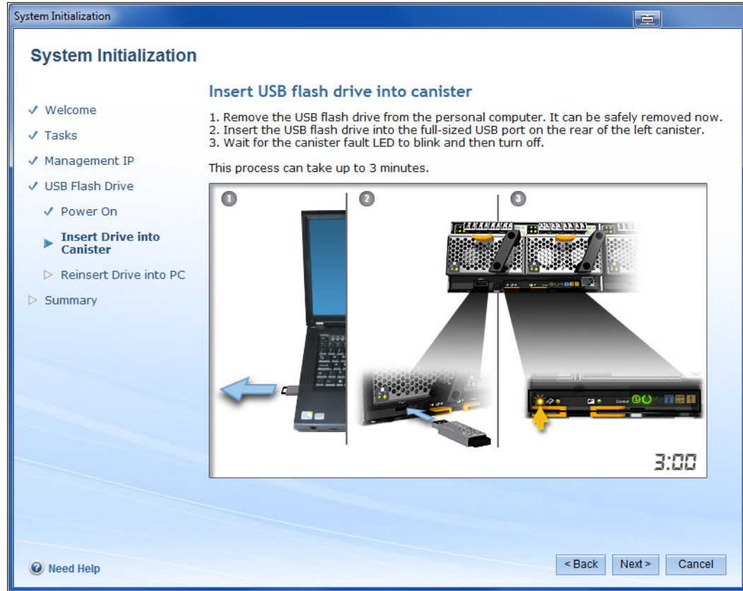
Figure 4-11 InitTool Insert USB flash drive into canister
