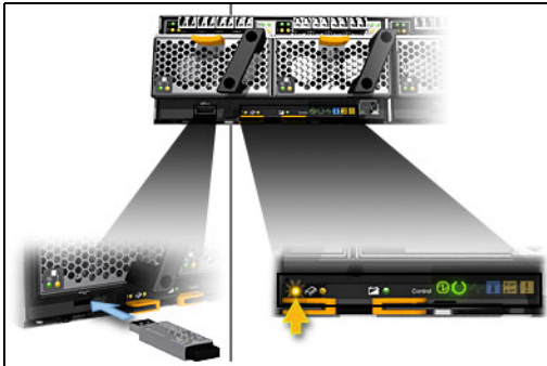
Figure 4-17 Inserting USB drive into canister and canister identify LED
