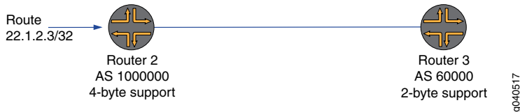
Figure 26: 4-Byte Capable Router Having a Peer Relationship with a 2-Byte Capable Router Using a 4-Byte AS Number
