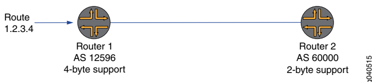
Figure 25: 4-Byte Capable Router Having a Peer Relationship with a 2-Byte Capable Router Using a 2-Byte AS Number
