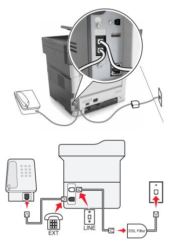
A Digital Subscriber Line splits your regular telephone line into two channels: voice and Internet. Telephone and fax signals travel through the voice channel, and Internet signals pass through the other channel. This way, you can use the same line for analog voice calls (including faxes) and digital Internet access.
