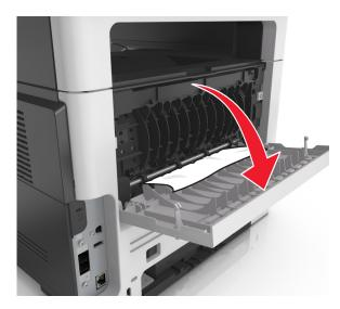
3 Firmly grasp the jammed paper on each side, and then gently pull it out.Note: Make sure all paper fragments are removed.
