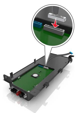
**9** Attach the ISP exterior cover at an angle by inserting the left hinges first.
