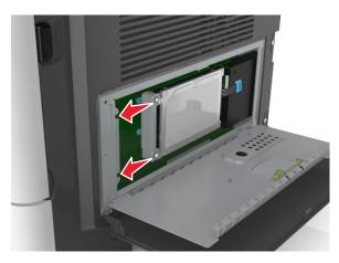
**d** Tighten the two screws.
