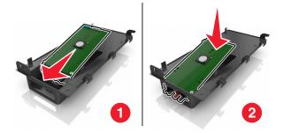
**6** Secure the ISP solution to the plastic bracket using the long screw.
