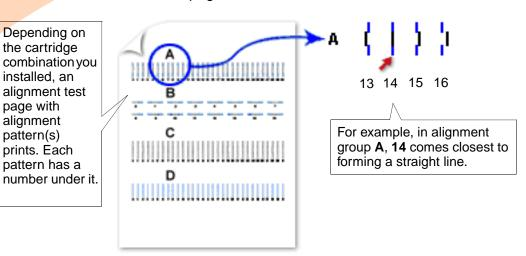
5 From each alignment group on the test page, find the number under the alignment pattern that comes closest to forming a straight line.
