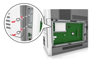
**4** Remove the printer hard disk.
