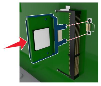
**Warning—Potential Damage:** Improper installation of the card may cause damage to the card and the controller board.
