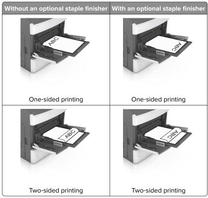
• There are different ways of loading letterhead depending on whether an optional staple finisher is installed or not.
