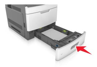
**8** From the printer control panel, set the paper size and paper type in the Paper menu to match the paper loaded in the tray.
