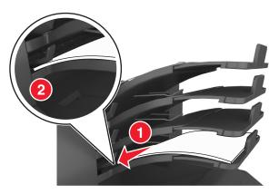
Note: If the paper is not under the bin arm, then a jam occurs due to an overfilled bin.
