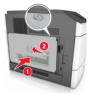
**6** Tighten the screws on the shield.
