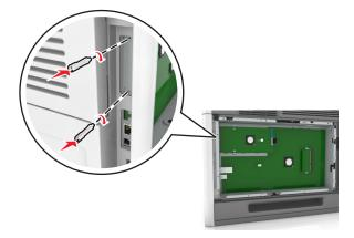
**10** Tighten the thumbscrew that is attached to the ISP.
