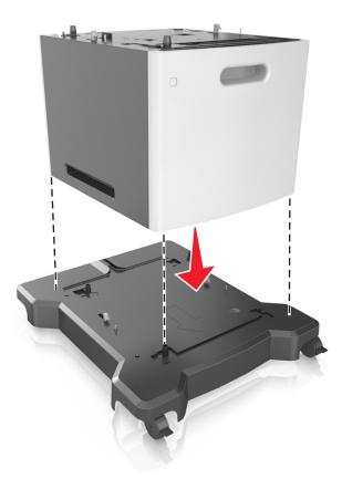
8 Align the printer with the tray, and then slowly lower the printer into place.Note: Optional trays lock together when stacked.
