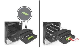
Note: Use the arrows on the side of the printer as a guide.
