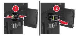
${\bf 3}~$  Lift the staple guard, and then remove the loose staples.
