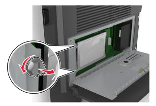
**3** Unplug the printer hard disk interface cable from the receptacle in the controller board, leaving the cable attached to the printer hard disk. To unplug the cable, squeeze the paddle at the plug of the interface cable to disengage the latch before pulling the cable out.
