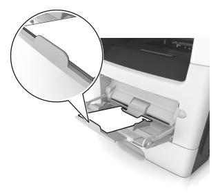
• Load letterhead faceup with the top edge entering the printer first. For two-sided (duplex) printing, load letterhead facedown with the bottom edge entering the printer first.
