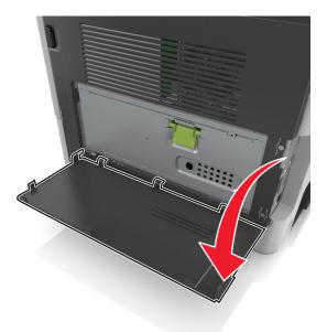
**2** Open the controller board shield using the green handle.
