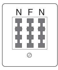
Connect the printer to any of the N ports.
