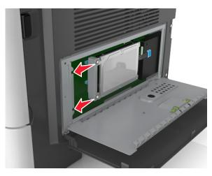
**d** Tighten the two screws.
