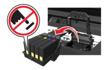
**3** Wipe the printhead contacts and the contacts inside the printhead carrier using a clean, lint-free cloth.
