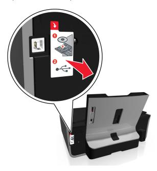
2 Firmly plug the square end of the USB cable into the back of the printer.
