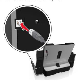
**3** Firmly plug the rectangular end of the USB cable into the USB port of the computer.
