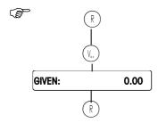
To use the "Calculating the change function", you only have to conclude the sale by the following sequence of keystrokes, the key R replaces the key \*\*
