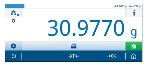
After a short period of time, the weighing pan is stable. The unstability symbol **O** disappears and the value in the weighing value field becomes dark blue again.
