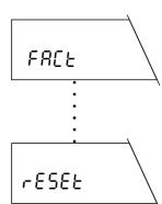
The next menu option appears in the display. Each time the « > » key is pressed, the balance switches to the following menu option.
