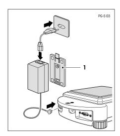
If you wish to work with the holder (1) supplied with the AC adapter: Attach the holder with two screws to a suitable, sufficiently stable area (e.g. on the wall or the underside of a bench top). Press the AC adapter into the holder.
