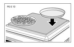
Place the additional weighing container on the weighing pan next to weighing containers already tared.
