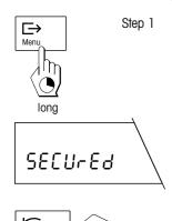
If "secure" is selected in the menu, "secure" appears when it is reentered (initiated by the menu key). If you do not press the « $\backsim$ » key for more than 3 seconds, the balance automatically returns to the weighing mode (menu remains blocked).
