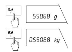
You can use the «S» key at any time to switch the display between the piece number display, weighing unit 1 and weighing unit 2.
