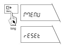
Press the **Menu**» key and keep it pressed until the balance switches to the menu.
