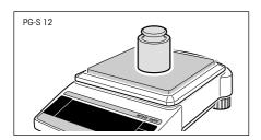
Place the requested weight in the middle of the weighing pan.
