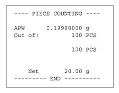
If a printer is connected to your balance, the reference weight, the reference piece number, the total piece count as well as the net weight of the total piece count are printed out.
