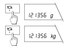
You can use the «S» key at any time to switch the display between percent display, weighing unit 1 and weighing unit 2.
