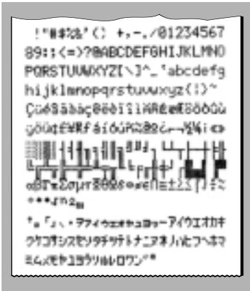
The GA42 is equipped with a self-test which automatically prints out the character set of the printer.
