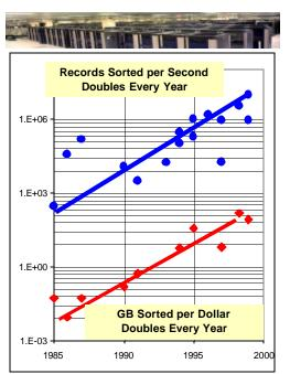
Figure 3: Top: a picture of the 6,000 node computer at LANL. Bottom: Scaleabilty of computer systems on the simple task of sorting data. Sort speed and sorting priceperformance has doubled each year over the last 15 years. This is progress is partly due to hardware and partly due to software. than creating it automatically.
