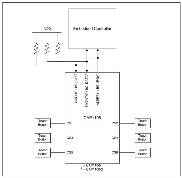
FIGURE 5-1: System Diagram for CAP1106
