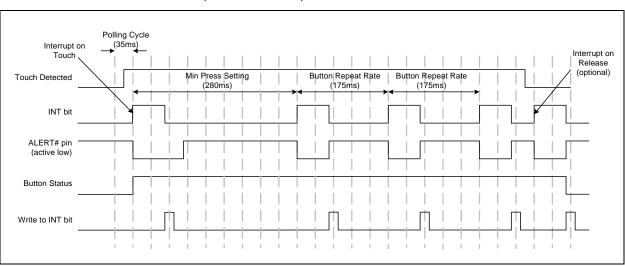
FIGURE 5-2: Sensor Interrupt Behavior - Repeat Rate Enabled
