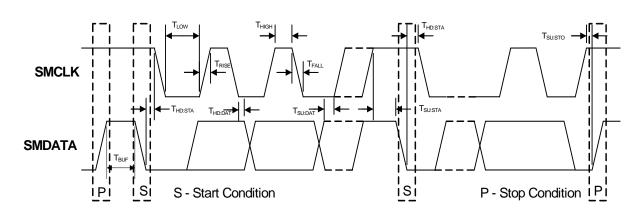
FIGURE 4-1: SMBus Timing Diagram
