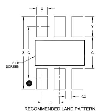
Units **MILLIMETERS Dimension Limits** MIN MOM MAX Contact Pitch Ε 0.95 BSC Contact Pad Spacing С 2.80 Contact Pad Width (X6) Χ 0.60 Contact Pad Length (X6) Υ 1.10 G 1.70 Distance Between Pads Distance Between Pads GX 0.35 Overall Width Z 3.90
