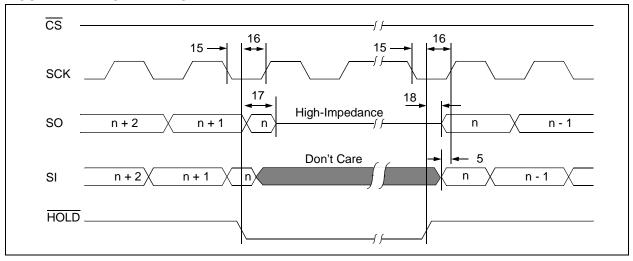
FIGURE 1-2: SERIAL INPUT TIMING (SPI MODE)
