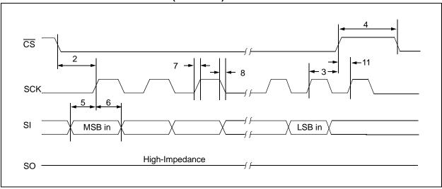
FIGURE 1-3: SERIAL OUTPUT TIMING (SPI MODE)
