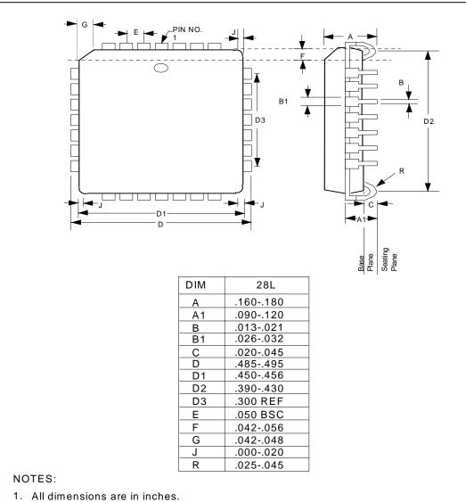
2. Circle indicating pin 1 can appear on a top surface as shown on the drawing or right above it on a beveled edge.
