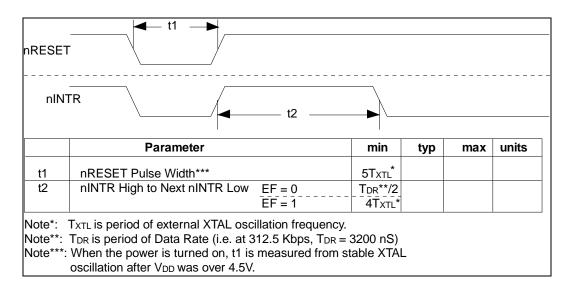
Figure 8.13 - RESET AND INTERRUPT TIMING
