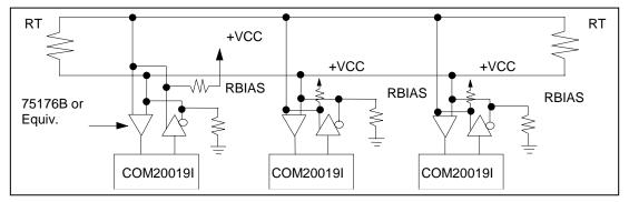
Figure 5.4 - COM20019I NETWORK USING RS-485 DIFFERENTIAL TRANSCEIVERS
