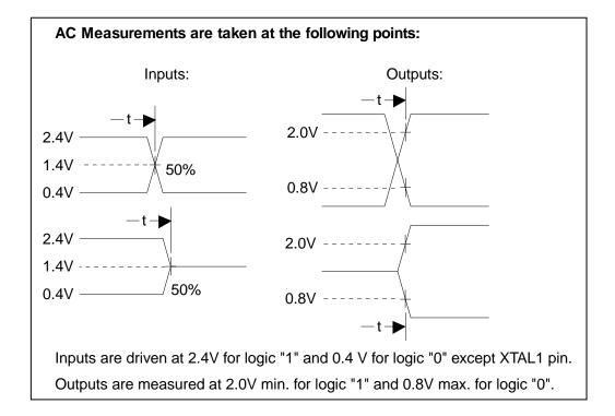
Figure 7.1 - AC MEASUREMENTS
