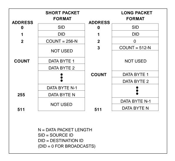
Figure 6.2 - RAM BUFFER PACKET CONFIGURATION
