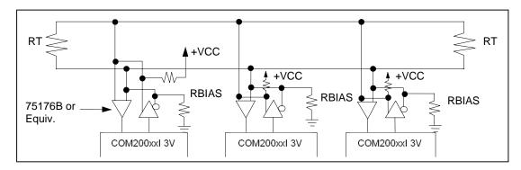
Figure 5 - COM20020I 3V Network Using RS-485 Differential Transceivers
