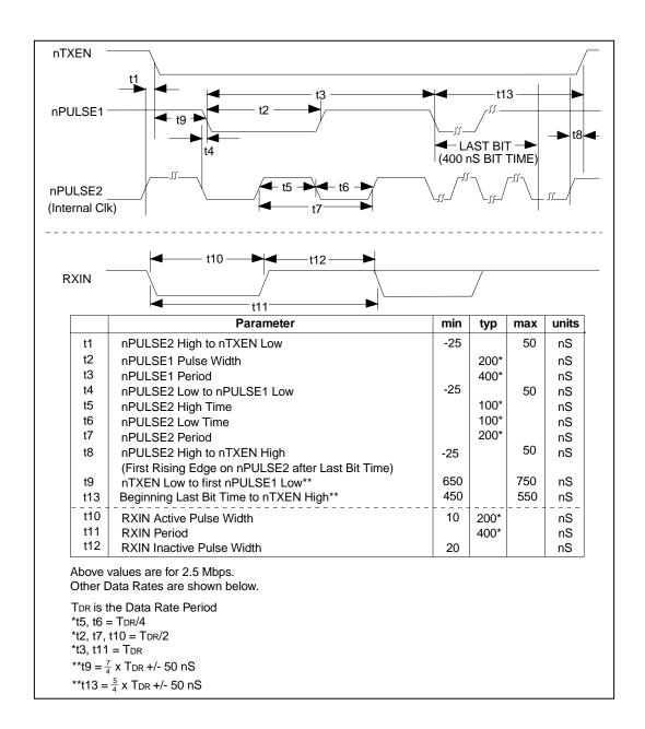
Figure 24 – Backplane Mode Transmit or Receive Timing (THESE SIGNALS ARE TO AND FROM THE DIFFERENTIAL DRIVER OR THE CABLE)
