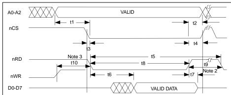
CASE 1 PLCC Package: Must be RBUSTMG bit = 0, TQFP Package: Must be BUSTMG pin = HIGH and RBUSTMG bit =0
