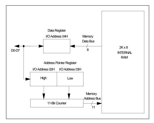
Figure 8 – Sequential Access Operation
