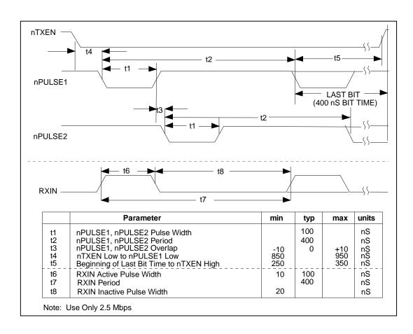
Figure 23 – Normal Mode Transmit Or Receive Timing (These signals are to and from the hybrid)
