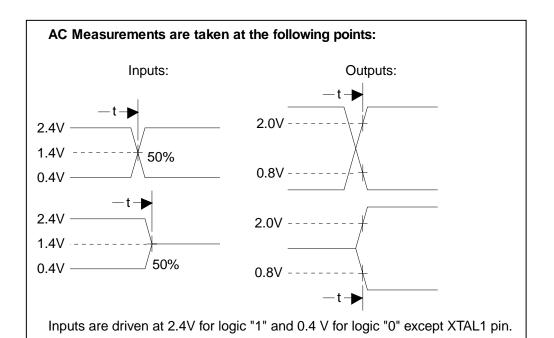
Outputs are measured at 2.0V min. for logic "1" and 0.8V max. for logic "0".
