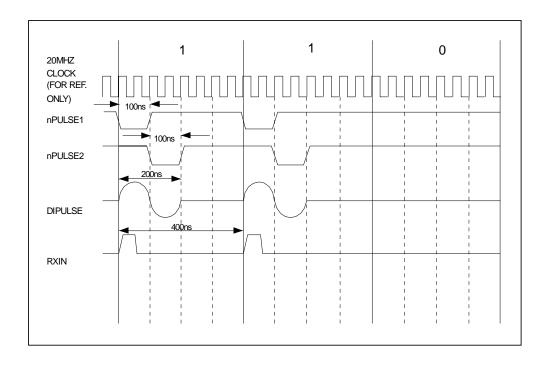
Figure 6 - Dipulse Waveform For Data Of 1-1-0
