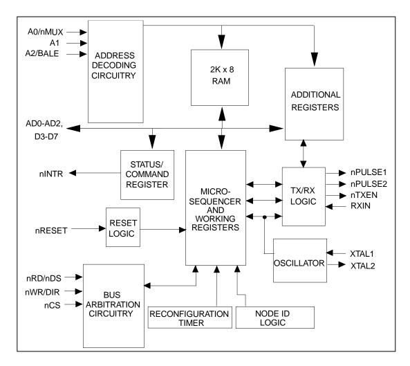
Figure 7 - Internal Block Diagram
