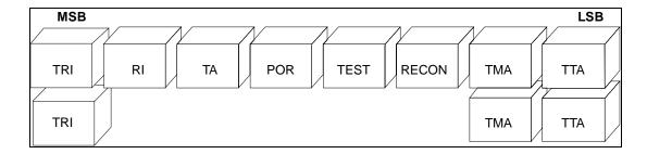
Figure 10 - Command Chaining Status Register Queue
