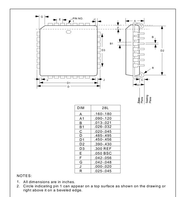
Figure 27 - 28 Pin PLCC Package Dimensions
