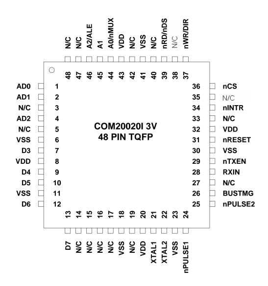
NOTE: BUSTMG pin is only TQFP package
