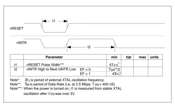
Figure 26 - Reset And Interrupt Timing
