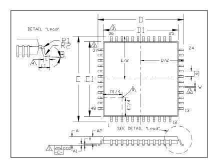
Figure 28 - 48 Pin TQFP Package Outline
