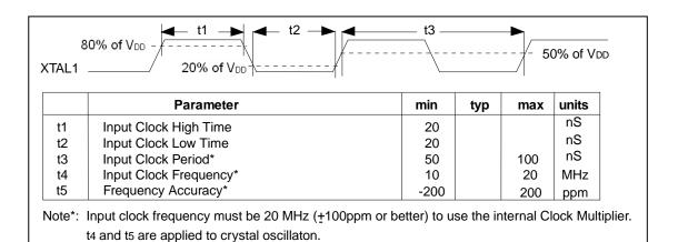
Figure 25 - TTL Input Timing On XTAL1 Pin
