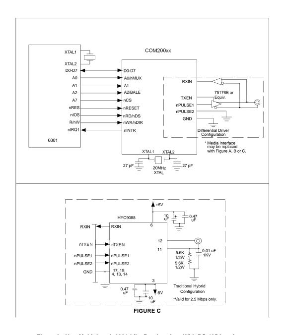
Figure 3 - Non-Multiplexed, 6801-Like Bus Interface With RS-485 Interface
