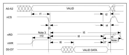
CASE 2 PLCC Package: Must be RBUSTMG bit = 1, TQFP Package: Must be BUSTMG pin = LOW or RBUSTMG bit =1
