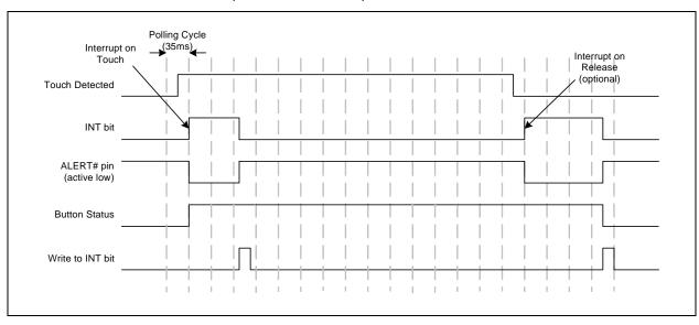
FIGURE 5-3: Sensor Interrupt Behavior - No Repeat Rate Enabled
