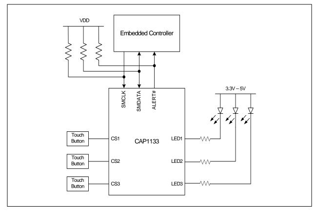
FIGURE 5-1: System Diagram for CAP1133
