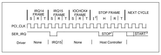
Note 1: H=Host Control; R=Recovery; T=Turn-Around; S=Sample; I=Idle
