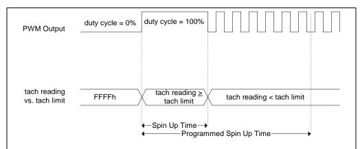
**Note**: When Spin Up Reduction is enabled (SUREN), the Spin Up time will be less than or equal to the programmed time for Spin Up. Once the tachometer(s) associated with a PWM output are operating within the programmed limits or the Spin Up time expires, whichever comes first, the PWM output is reduced to the calculated duty cycle.
