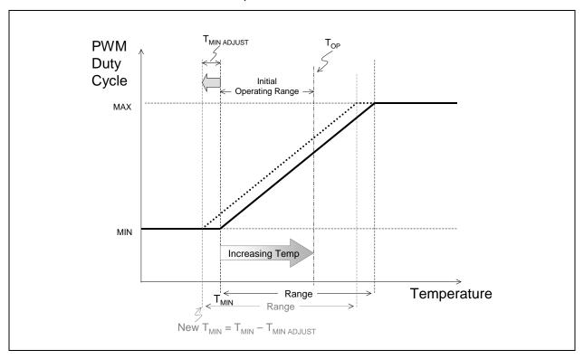
FIGURE 20-13: AMTA ILLUSTRATION, ADJUSTING MINIMUM TEMPERATURE
