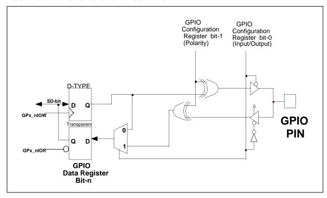
FIGURE 10-1: GPIO FUNCTION ILLUSTRATION
