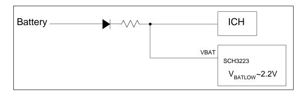
Note that the battery voltage of 2.2V nominal is at the VBAT pin of the device, not at the source.
