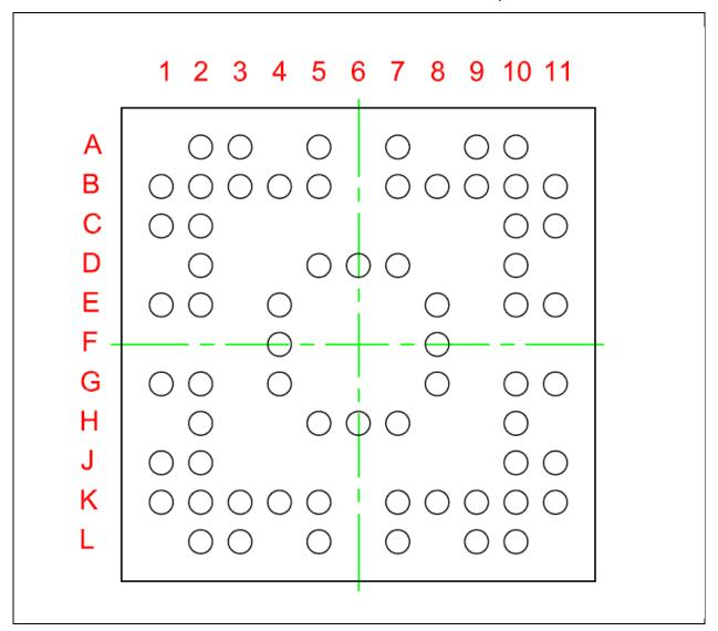
This is a 64-ball 6mm x 6mm package, with ball pitch of 0.5mm. However, the sparse 0.5mm pitch ball array allows 0.65mm trace routing rules. For a specific recommendation, see the drawing in Section 27.0, "Package Outline," on page 188.
