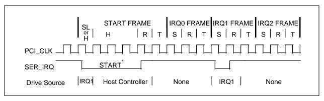
Note 1: H=Host Control; R=Recovery; T=Turn-Around; SL=Slave Control; S=Sample
