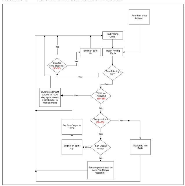
When in Auto Fan Control Operating Mode the hardware controls the fans directly based on monitoring of temperature and speed.
