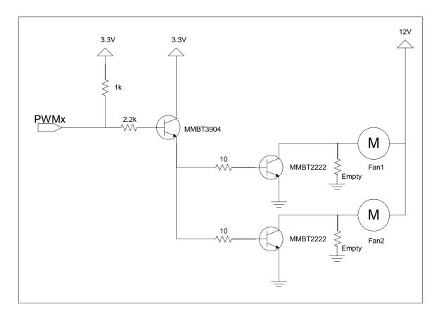
FIGURE B-2: FAN DRIVE CIRCUITRY FOR LOW FREQUENCY OPTION (APPLY TO PWM DRIVING ONE FAN)
