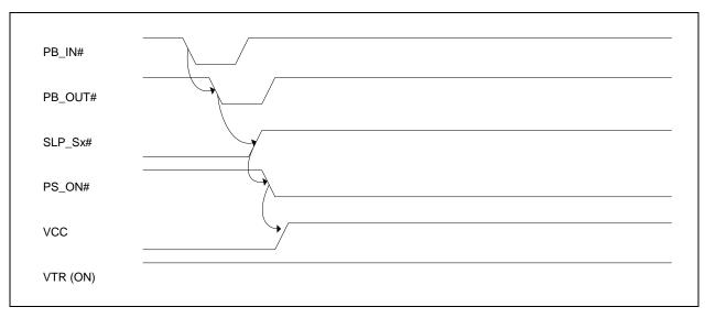
FIGURE 17-4: POWER SUPPLY AFTER POWER FAILURE (RETURN TO OFF)
