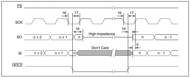
FIGURE 1-2: SERIAL INPUT TIMING
