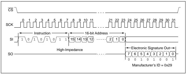
Driving  $\overline{\text{CS}}$  high after the 8-bit RDID command but before the Electronic Signature has been transmitted will still ensure the device will be taken out of Deep Power-Down mode. However, there is a delay  $T_{\text{REL}}$  that occurs before the device returns to Standby mode ( $I_{\text{CCS}}$ ), as shown in Figure 2-13.
