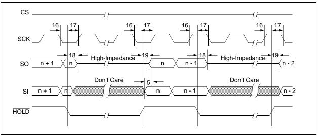
FIGURE 1-2: SERIAL INPUT TIMING
