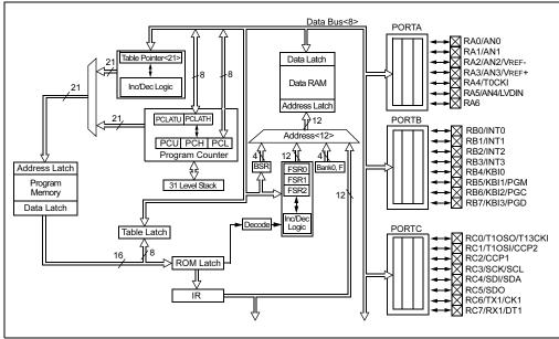
FIGURE 1-1: PICmicro<sup>®</sup> MCU DATA SHEET - BLOCK DIAGRAM (EXCERPT)
